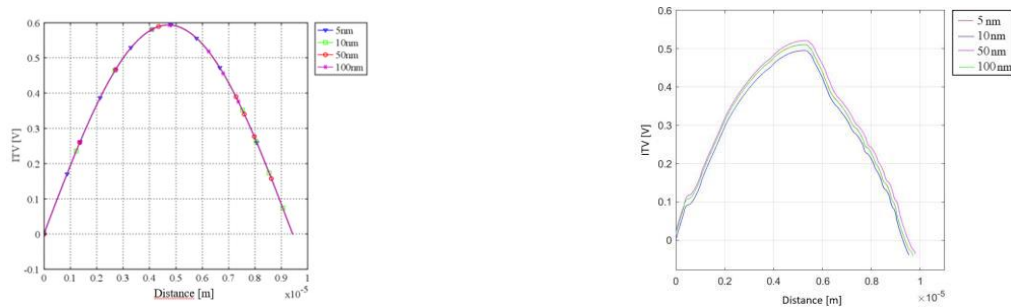
Fig. 5.4 ITV amplitude (absolute value) on the half of the cell contour for various membrane thicknesses within the range of 5 to 100nm for a) Circular cell_B and b) Realistic cell_B exposed to a low-frequency electric field [23]
