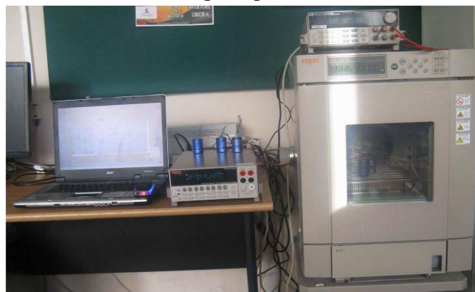
Fig. 4. 4 Measurement system with the supercapacitors subjected to testing.
