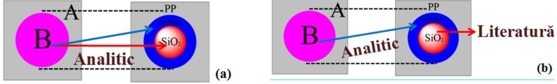
*Fig. 5.1.* Assigning the values of the electrical permittivity found for component B to the subdomains of the geometric model: CASE I (a) and CASE II (b).
