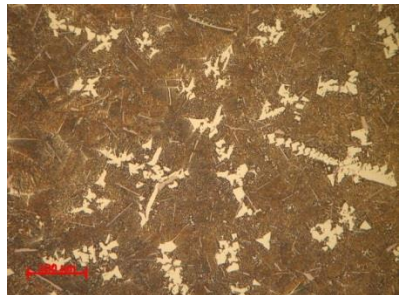
Fig 3.13. YPM4 alloy microstructure (200 ×)
