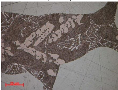
Fig 3.7. YSM4 alloy microstructure (900 ×)
