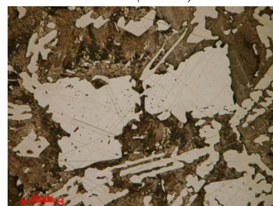
Fig. 3.14. YPM4 microaliat cu 1,0 % Mm (900 ×)
