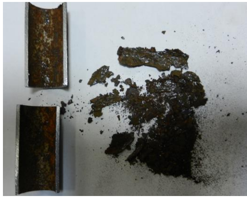
Figure 5. 18 Residue deposits on the inner surfaces of heat exchanger tubes.
