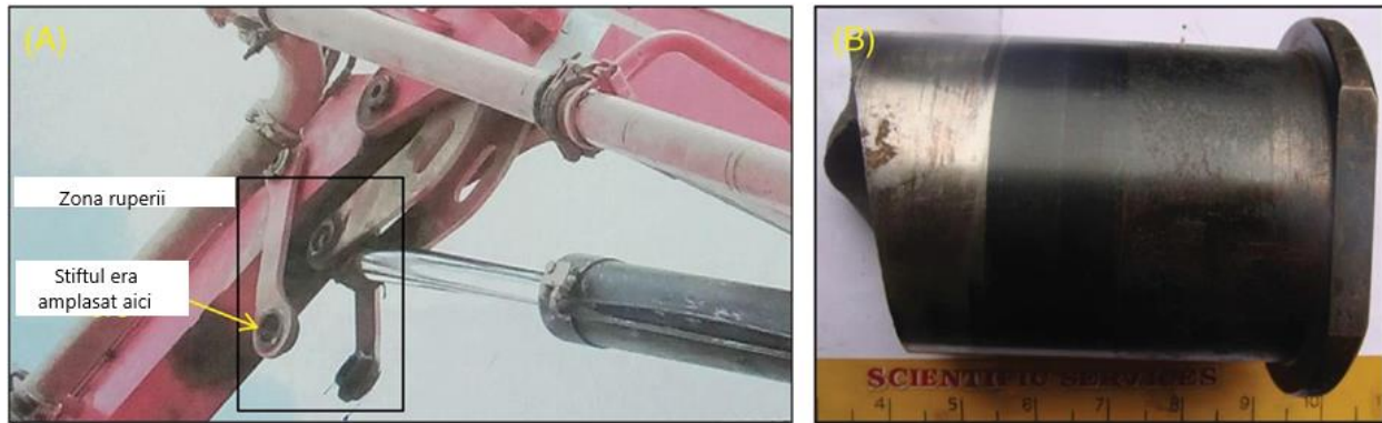
Figure 2. 16. (A) Location of the arm pin failure at the arm setter, (B) defective arm pin [137].
