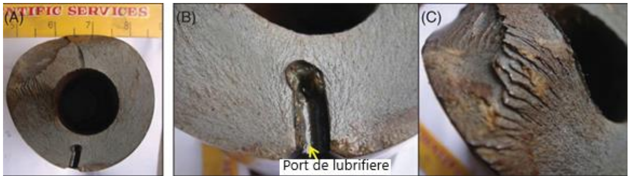
Figure 2.17. (A) Fracture surface of the arm pin, (B) initiation of chevron marks from the lubrication port indicating a brittle fracture, and (C) radial marks suggesting brittle fracture of the arm pin [137]
