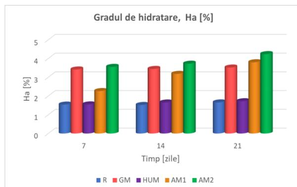
Figure 6.16 Variation of hydration over a period of 21 days in distilled water, at  $37^\circ\text{C}$ , for experimental samples
