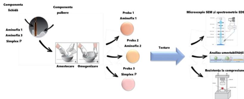
The figure below shows the process of obtaining experimental samples of bone cement, to which antimicrobial agents have been added.
