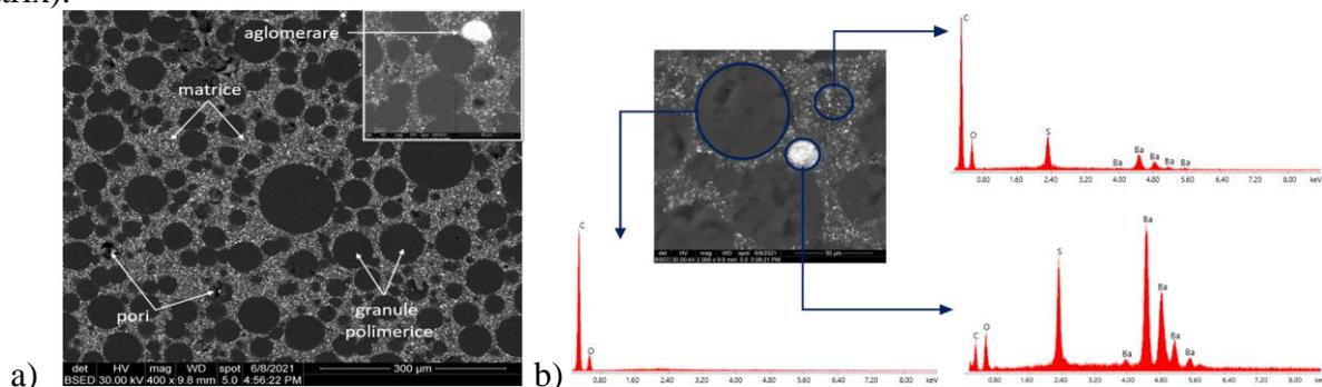
Figure 6.3. SEM image of the GM sample (400 X) a) and representative SEM image (2000 X) and EDX analysis performed on different areas for the GM sample
