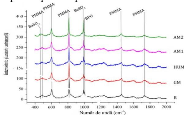
*Figure 6.12 Raman models collected on studied samples - made of PMMA-BaSO<sub>4</sub>-BPO as major components. The most intense strips were labeled and assigned to that component of bone cement*
