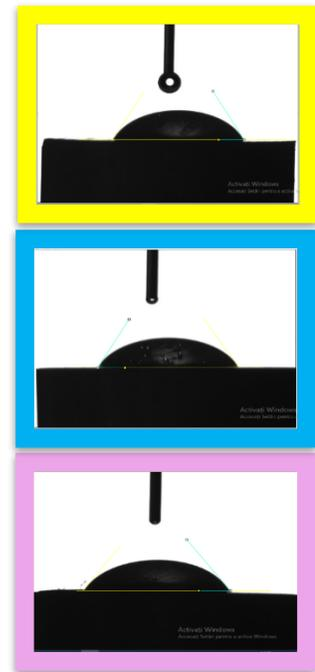
The contact angle values for the investigated samples were very close to each other ranging between 55 and 61 degrees. The results obtained indicate that the sample surfaces were hydrophilic. A hydrophilic surface reflects good wettability and adhesion, so better osseointegration. An optimal contact angle value for cell adhesion is approximately  $55^\circ$  [7,8], the closest value measured in this research being obtained in sample 3 ( $55.1^\circ$ ) followed by sample 1 and sample 2.
