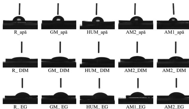
Figure 6.14 Appearance of droplets formed on the surface
