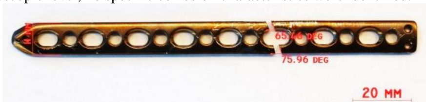
FIG. 4.11 Macrography of the LCP type explant
