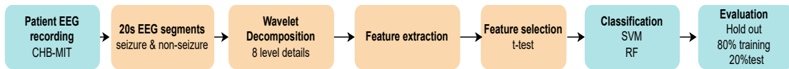
Fig. 3.2 Method for detecting epileptic seizures using features extracted from the detail coefficients of a 8 level Wavelet decomposition.
