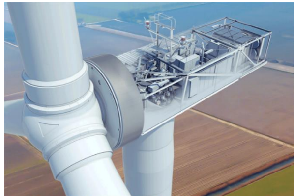
Figure no. 59. Nacelle image (inner structure) source: nacelle picture - Bing images
