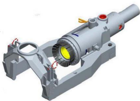
Figure no. 79. UCON system used to connect various devices when extracting oil from the bottom of the water at depths even over 6000 m.
