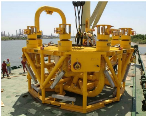
Figura nr. 77. Production Manifold (Source: Onesubsea – Cameron & Schlumberger company )
