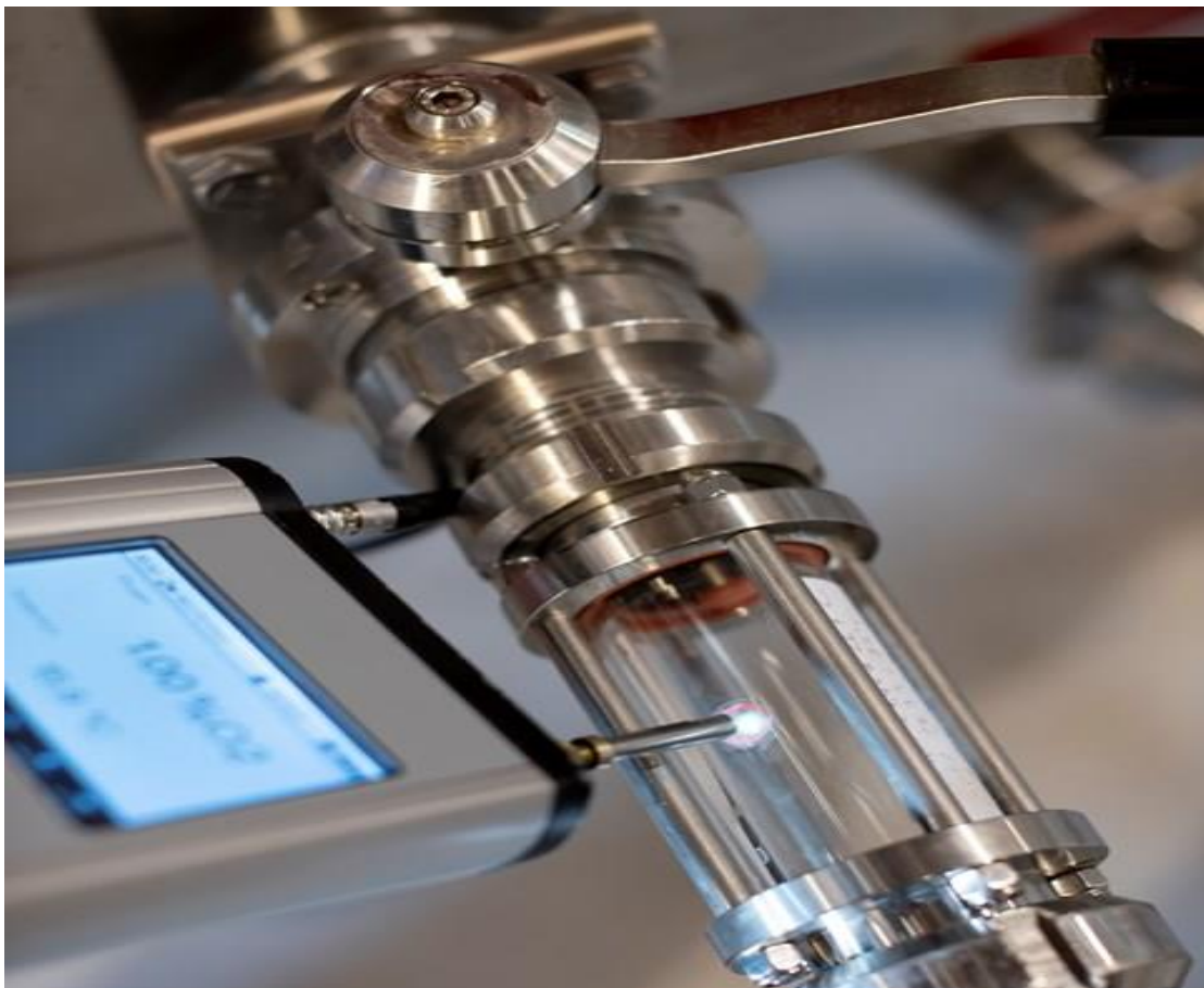
Fig. 16. How to measure the concentration of dissolved oxygen in water with the NomaSense portable oxygen meter
