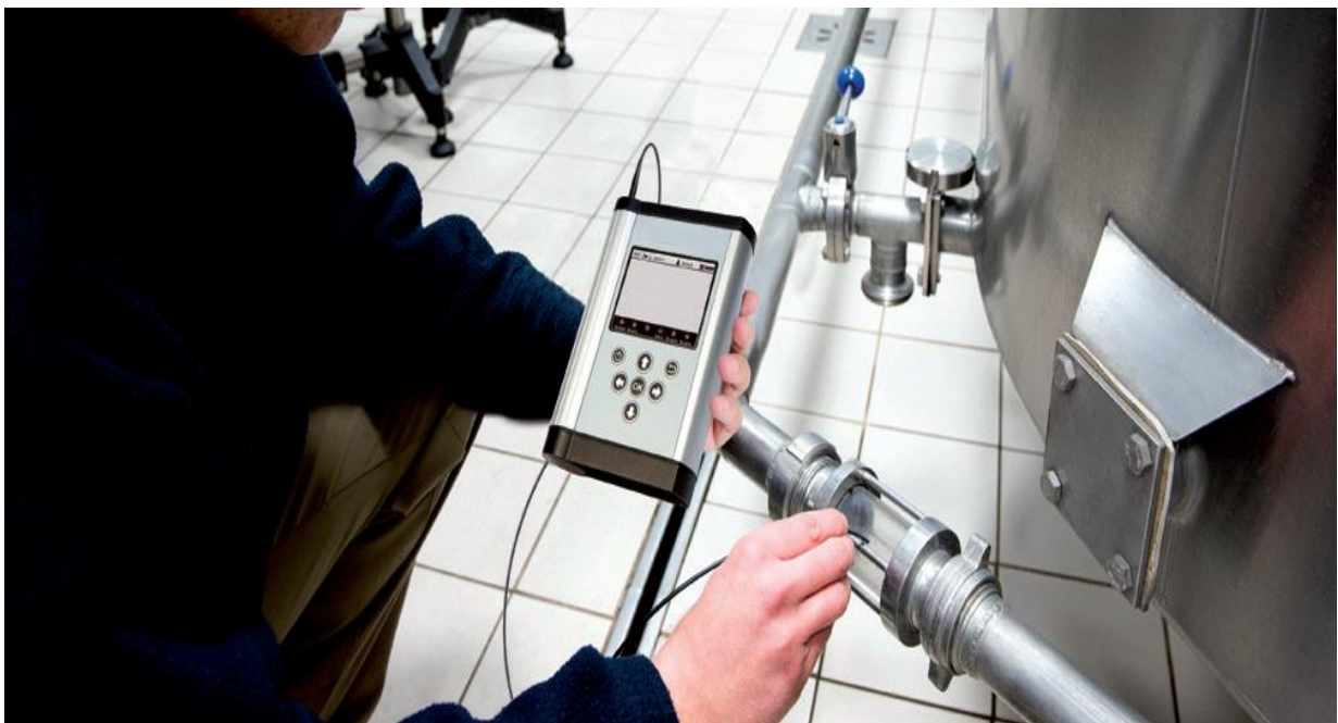
Fig. 14. Non-invasive device for measuring dissolved oxygen concentration
