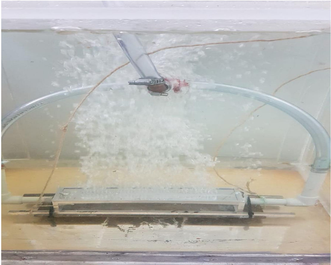
Fig. 21. Bubble curtain emitted by the fine bubble generator in operation
