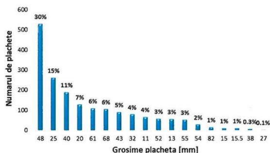
The analysis regarding the products made of 3003 plated aluminum alloy was performed for the period 01.11.2016 ÷ 31.10.2017. Data for this analysis were extracted from the Centralizer application. Figure 3.4 shows the structure of the plates made according to their thickness. Thus, most of the plates made (528) had a thickness of 48 mm and correspond to a cladding percentage of 10%.
