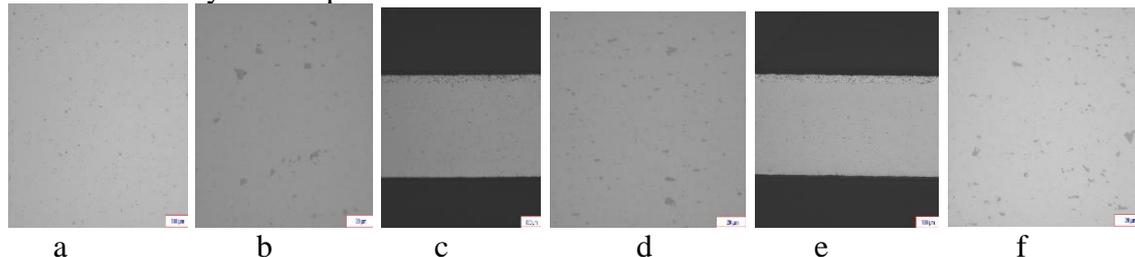
FIG. 5.18- The microstructural aspect of the specimens from 3003 plated with 4045, in state O, unattached, sections and magnifying powers (a, c, e x100; b, d, f- x500; a, b- flat section; c, d, cross section; e, f- longitudinal section)
