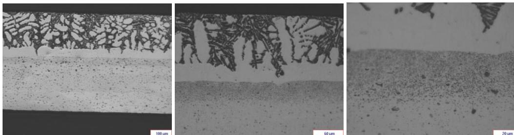
FIG. 5.22- The microstructural aspect of the brazing layer of alloy 3003 with alloy 4343, at different magnifying powers
