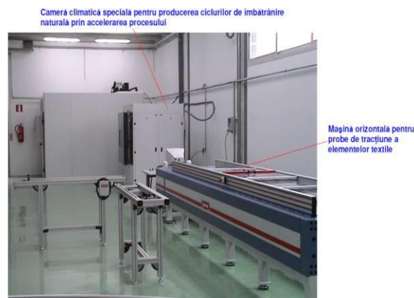
Picture 2.2. Indoor area of the Safety Elements Laboratory for static resistance tests and accelerated ageing tests.
