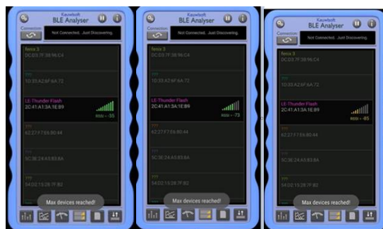
Fig. 5.30. RSSI level of bluetooth headphones at different distances
