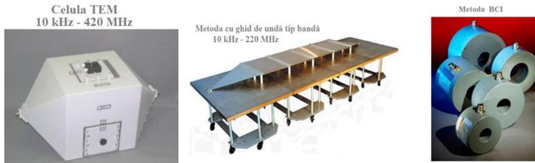
Figure 6.2: ISO 11452 test methods: TEM cell, stripline method, BCI method [19]
