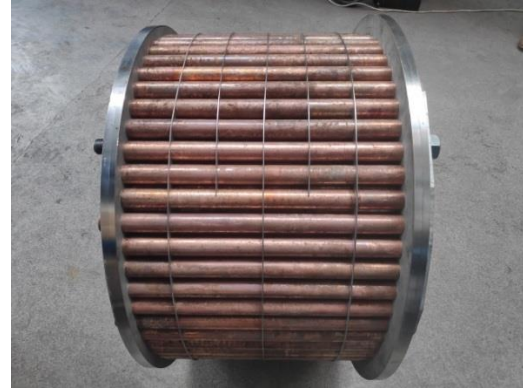
Figure 17 - The heat exchanger assembly before the welding process
