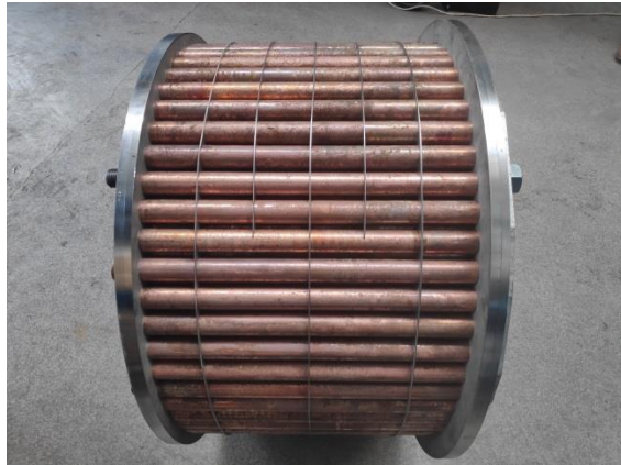
Figure 9 - Side and frontal view of the heat exchanger assembly
