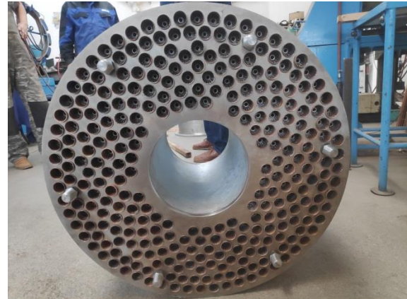
Figure 9 - Side and frontal view of the heat exchanger assembly
