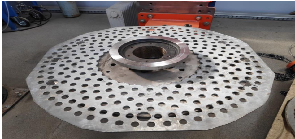
Figure 24 – Aluminum template "Amisab" designed to achieve uniform reinforcement of the part
