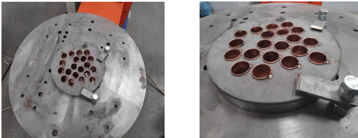
Figure 10 – The test piece used to perform robotic welding of copper pipes
