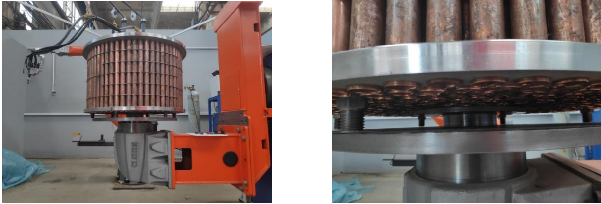
Figure 19 - Fixing and centering the part with the "Amifix" device on the robotic system table
