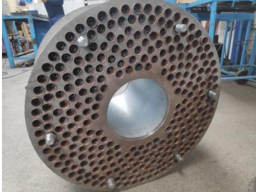
Figure 17 - The heat exchanger assembly before the welding process
