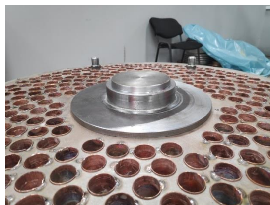
Figure 18 - The final version of the "Amifix" centering and fixing device
