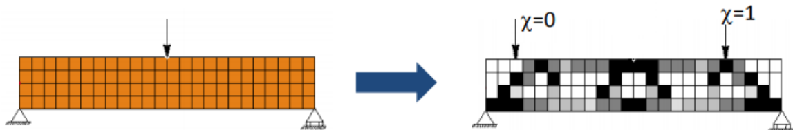
Fig. 4.6. Geometric representation of the structure [34]
