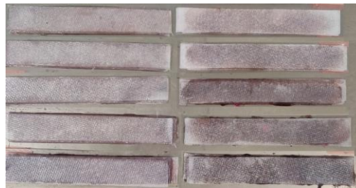
Figure 6.1. Flexural sample manufacturing with embedded microencapsulated healing system
