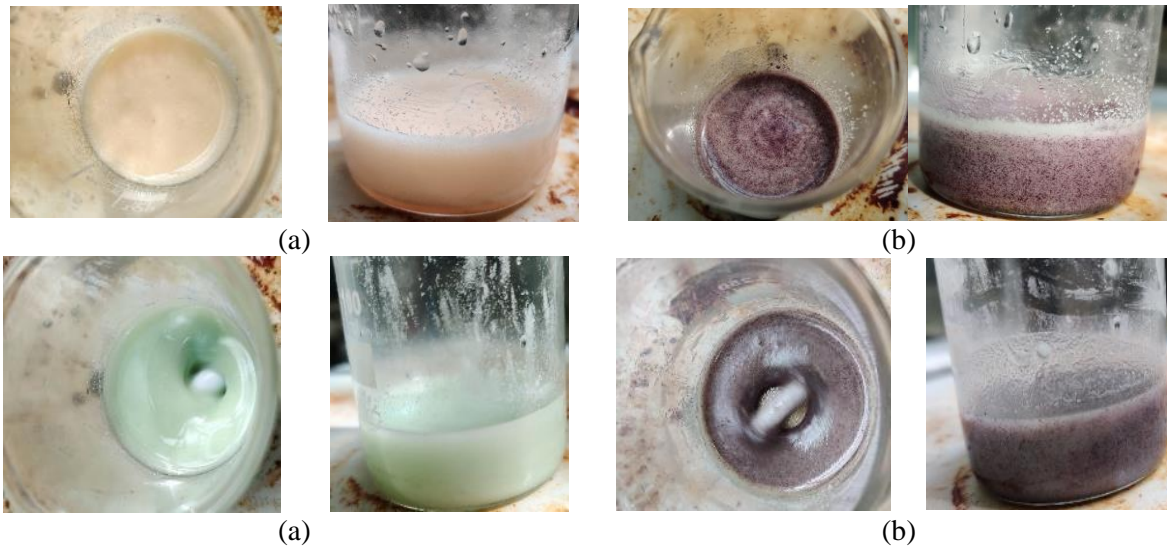
Figure 3.13. Realizing the mixture between Resoltech resin 1050/1058, with a) PUF-DCPD microcapsules and b) Grubbs catalyst by magnetic dispersion
