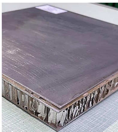
Fig. 4.1 Ol-Al-Al Honeycomb-Ol plate
