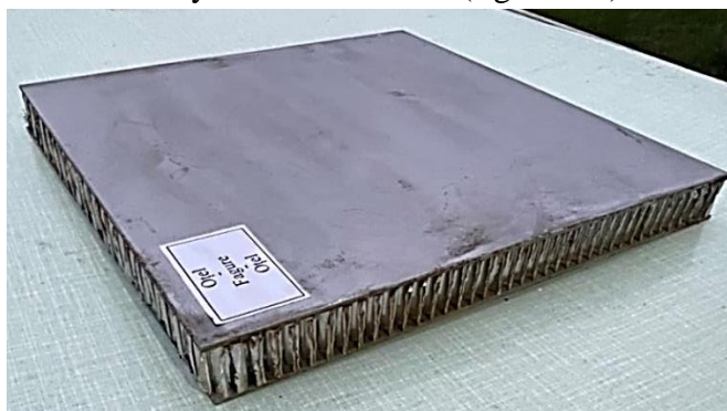
Fig. 4.3 OI-Al Honeycomb-OI plate
