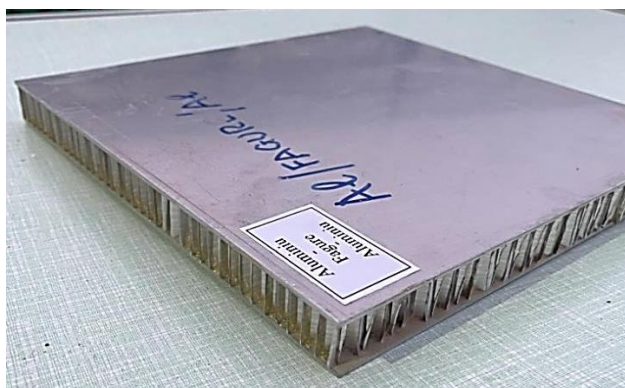
Fig. 4.2 Al-Al Honeycomb-Al plate
