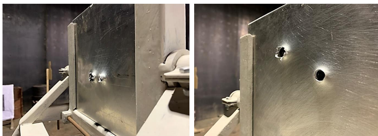
Fig. 4.7 OI-Al-F-Al plates - 2 x 7.62 mm - rear view
