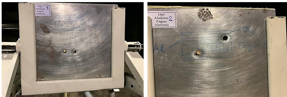
Fig. 4.6 OI-Al-F-Al plates - 2 x 7.62 mm - impacted front view
