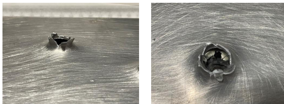
Fig. 4.10 Appearance of the hole after impact OI-Al-F-Al plate - experimental testing
