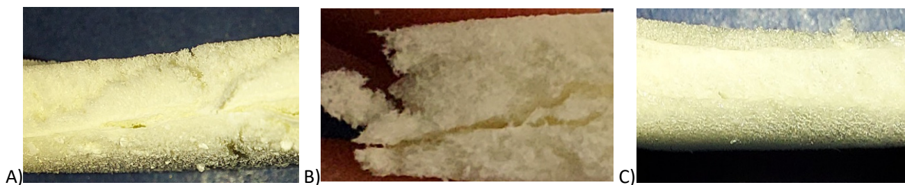
Figure 12 Cross section images of 10HA-90KNN-CSL 1.5 (A), 50HA-50KNN-CSL 3 (B), 90HA-10KNN-CSH 1.5 (C) scaffolds, after lyophilization
