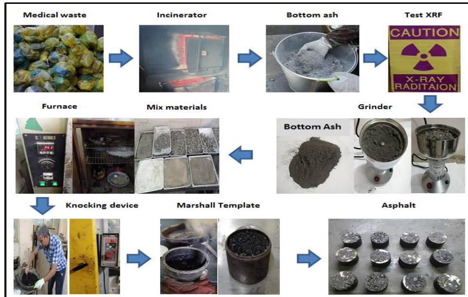
Figure 4.1 The stages of converting medical waste into bottom ash and mixing it with the asphalt mixture[106]
