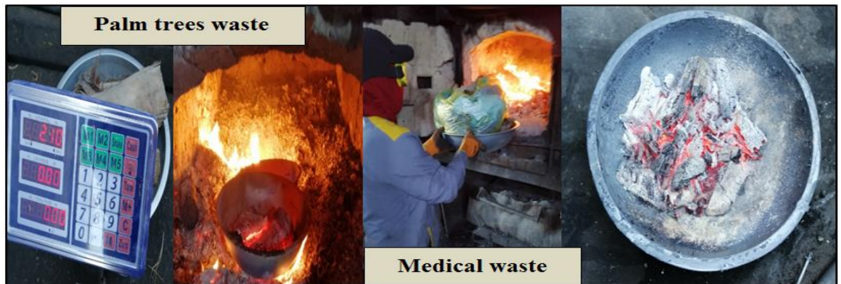
Figure 5.7 Burning medical waste and palm waste in the medical incinerator
