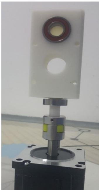
Fig. 9.6. Assembling the engine with the shaft
