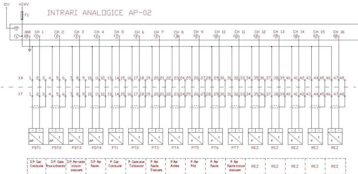
Figure 3.23. Diagram of gas turbine instrumentation for basic parameters
