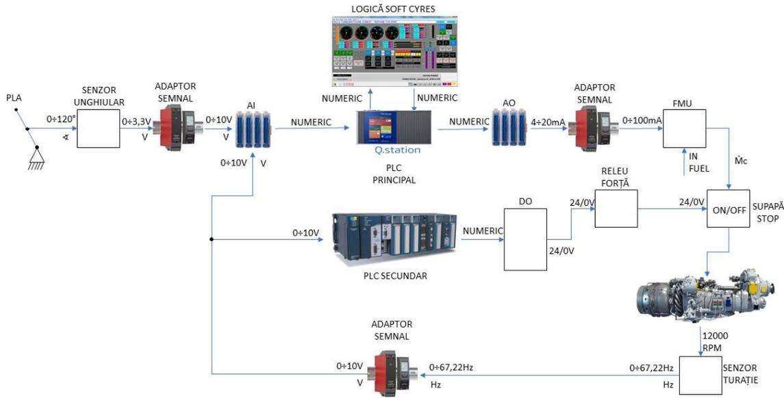
Figure 5.6. Block diagram for the mode regulation line together with the feedback and the NTP emergency stop line separated by a secondary safety PLC
