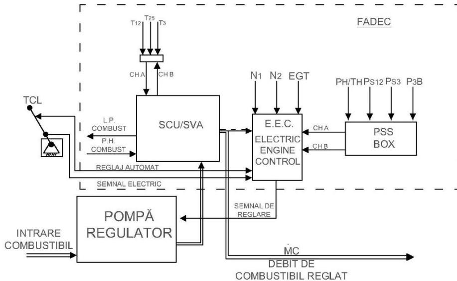
Figure 1.16. Electro-hydraulic fuel regulation system with FADEC electronic assistance [41]
