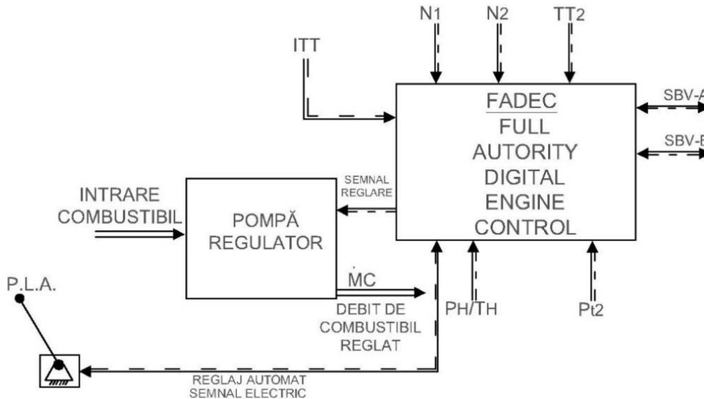
Figure 1.14. Electro-hydraulic fuel regulation system with FADEC electronic assistance [39]
