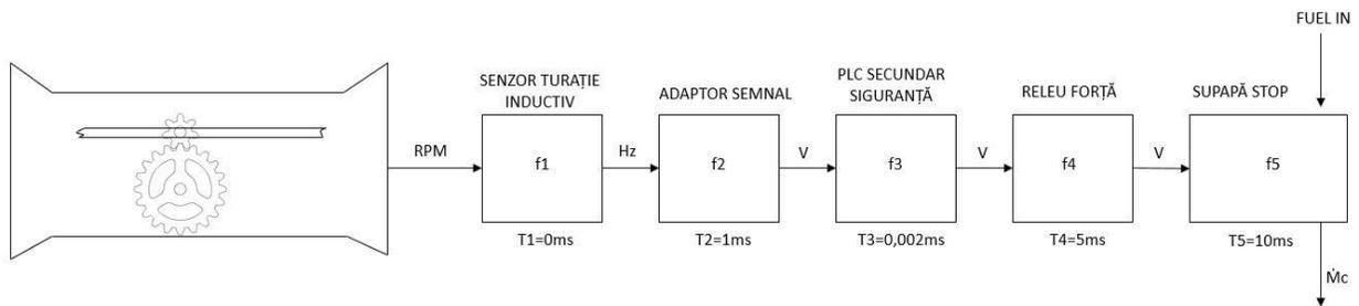
Figure 5.5. Logic diagram regarding delay times
