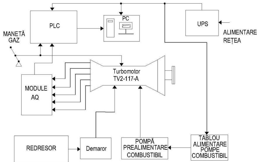
Figure 3.1. Block diagram of the classic gas turbine automatic regulation system together with the auxiliary installations
