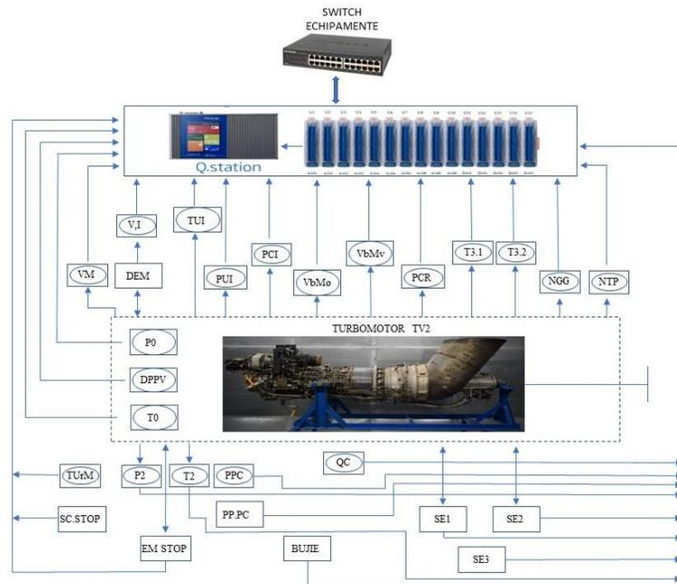
Figure 5.35. Instrumentation, command and control diagram for the TV2-117A gas turbine
