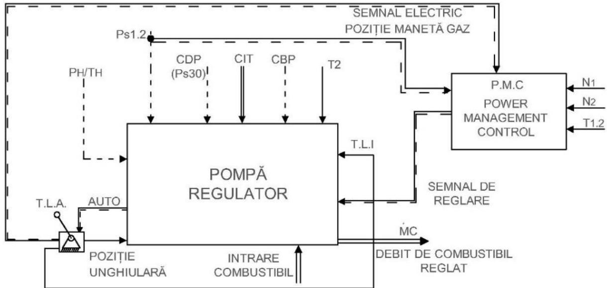
Figure 1.8. Hydromechanical fuel regulation system with electronic assistance [33]
