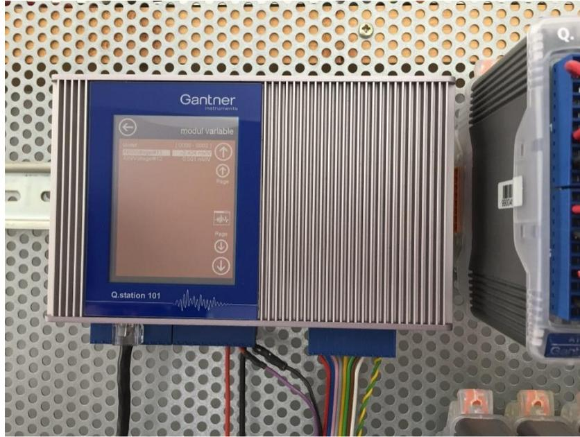
Figure 5.11. Data acquisition and control system consisting of Q.station and Q.series
