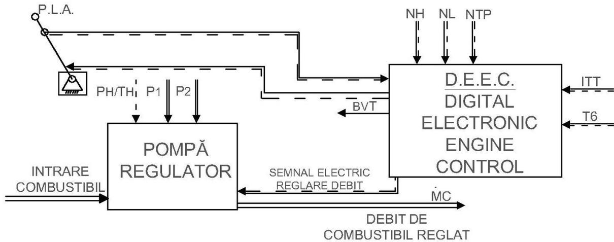
Figure 1.12. Electro-hydraulic fuel regulation system with D.E.E.C. electronic assistance. [37]
