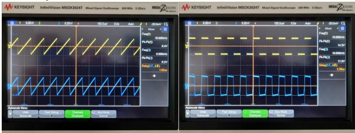
Figure 5.40. Ramp signal simulation Figure 5.42. Step signal simulation
