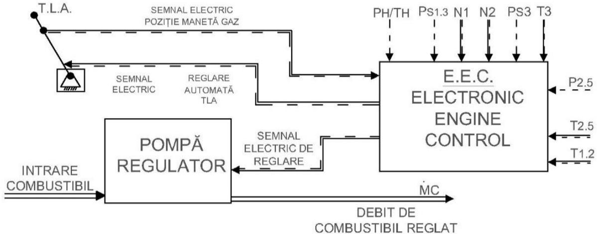
Figure 1.10. Electro-hydraulic fuel regulation system with electronic assistance E.E.C. [35]
