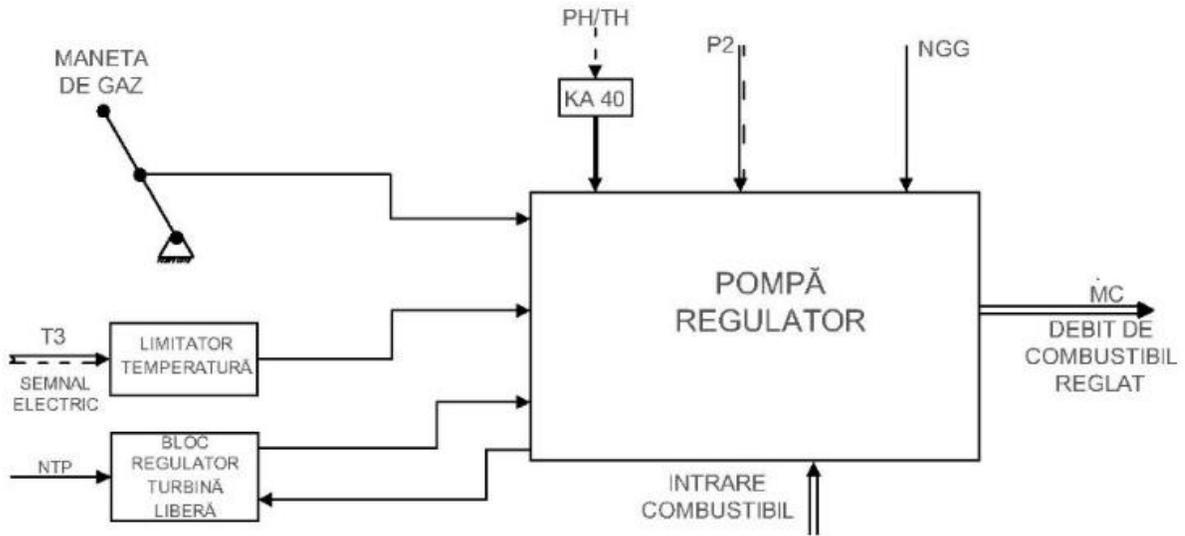
Figure 1.6. Hydro-mechanical fuel control system without electronic assistance [31]
