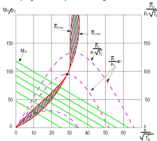
Figure 2.34. Mechanical characteristic of low-pressure air starter [3,58]
