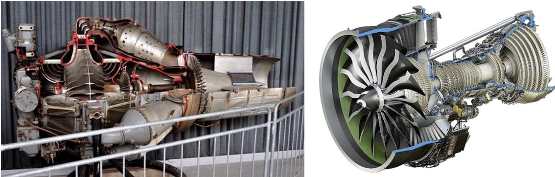
Figure 1.5. The RD45 turbojet engine, with a maximum thrust of 12 *TF* [8] The GE9X turbofan, with a maximum thrust of 50 *TF* [30]
