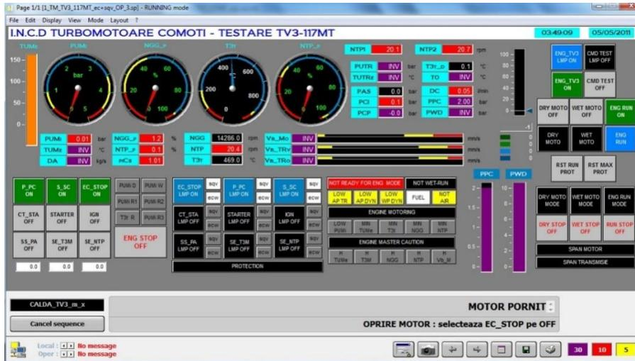
Figure 4.13. The operating panel for testing the gas turbine
