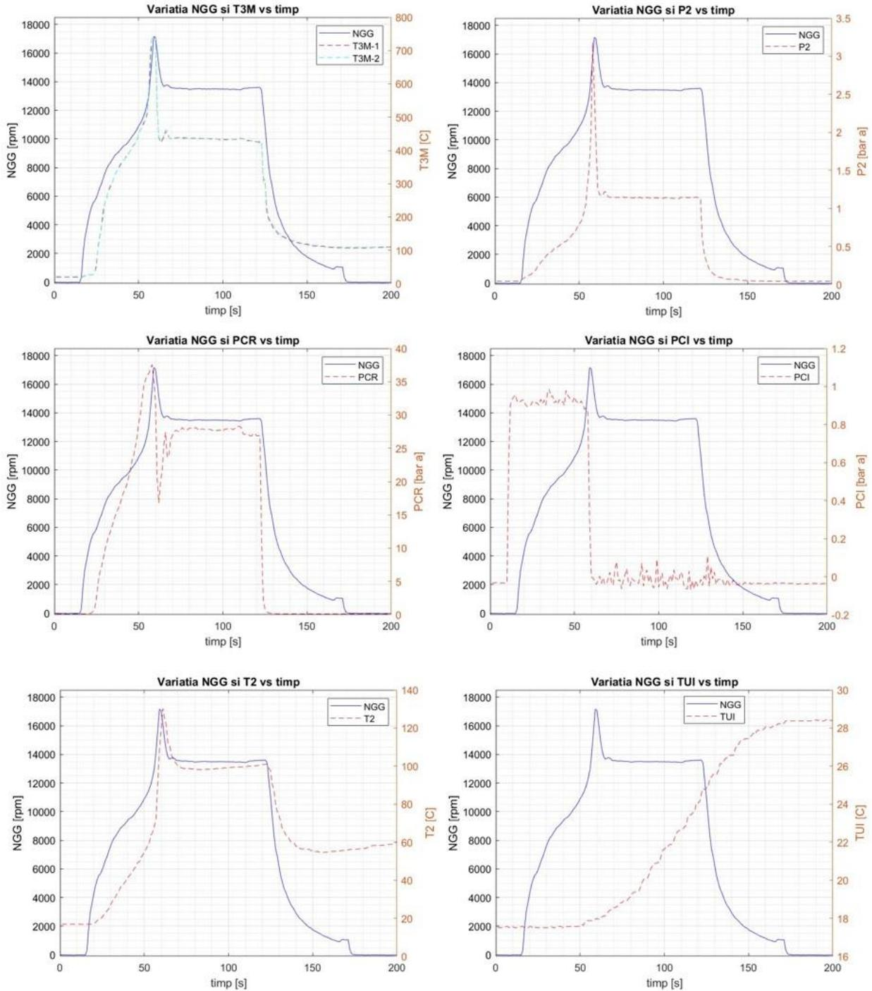
Figure 3.37. Average Combustion Chamber Temperature (T3M), After Compressor Pressure (P2), Ramp Fuel Pressure (PCR), Fuel Pressure (PCI), After Compressor Temperature (T2), Engine Inlet Oil Temperature (TUI) vs RPM gas generator (NGG) from Experiment No. 2
