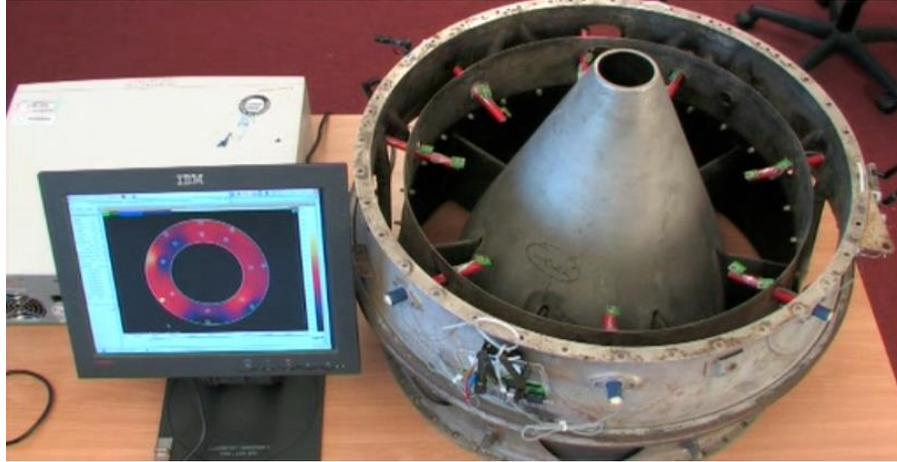
Figure 4.14. Feedback aid with prototype wireless instrumentation system [82]
