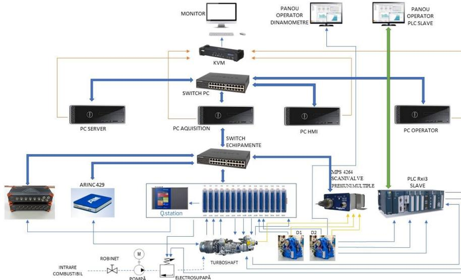
Figure 5.9. Block diagram of the system used in the configuration for engines with turboshaft
