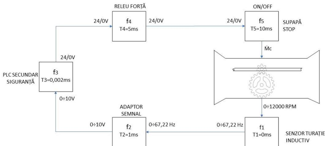
Figure 5.2. Block diagram of emergency stop line by NTP speed parameter
