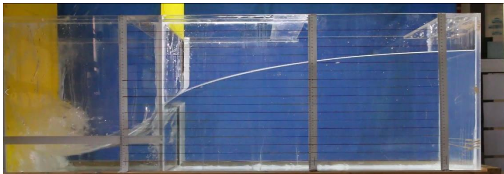
Figure 5.3 The experimental cases of dam breaking from the small section to the large section and vice versa at the specified static heights
