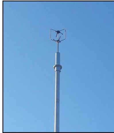
Figure A3.1 Ultrasonic anemometer type WindMaster 3 - testing and calibrating
