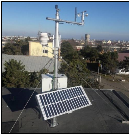
Figure A3.2 The hydrometeorological installation type WS-GP2 - testing and calibrating
