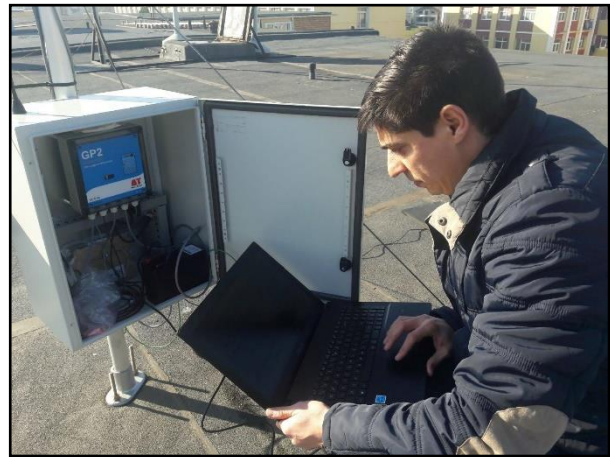
Figure A3.2 The hydrometeorological installation type WS-GP2 - testing and calibrating
