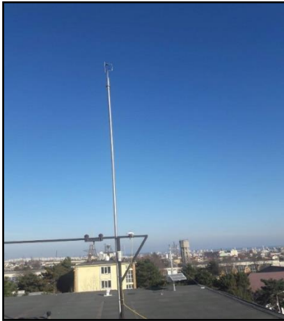
Figure A3.1 Ultrasonic anemometer type WindMaster 3 - testing and calibrating
