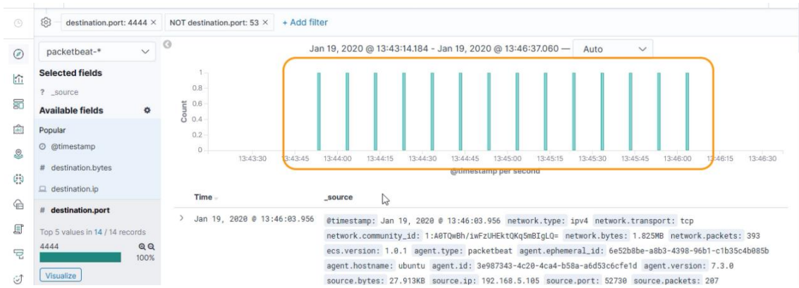
Figure 3.15 Anomaly detection based on time intervals between connections.
