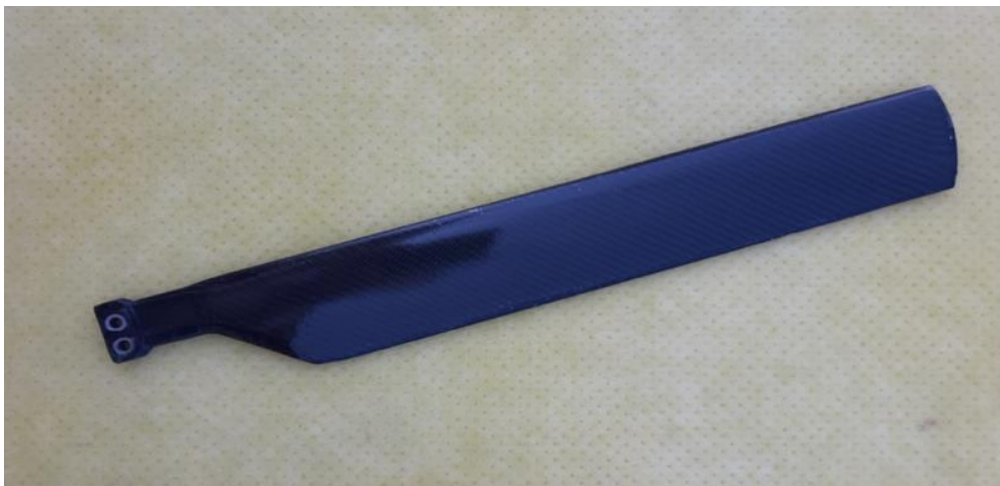
Fig. 7.1 The final composite tail rotor blade at a scale of 1:3
