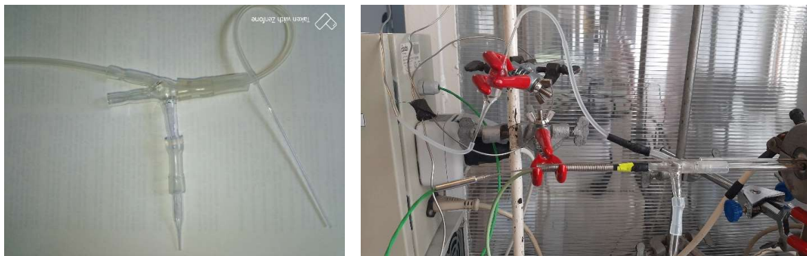
Fig. 2.8. The glass piece for introducing the reactant mixture and water into the reactor: on the left - T-Y piece with three inlets (top: water hose, middle: thermocouple, bottom: inlet for reactants mixture/hydrogen for regeneration) and one outlet. On the right - installation overview of the T-Y glass piece
