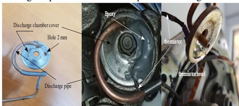
Figure 3-4: Discharge chamber cover
