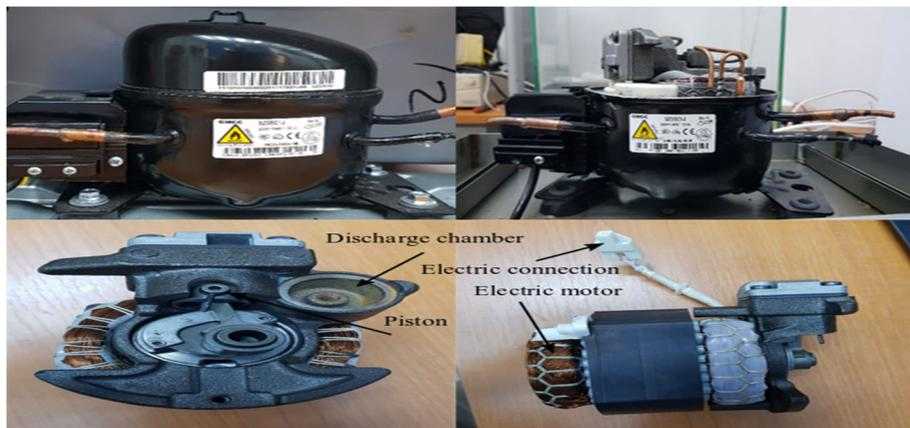
Figure 3-3: Internal component of the experimental compressor
