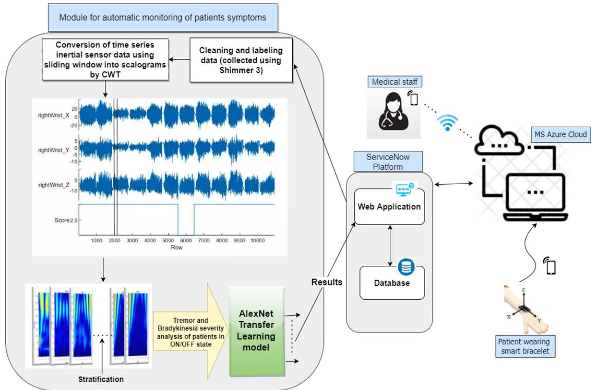
Figure 5.1: The block diagram of the proposed PD monitoring system.
