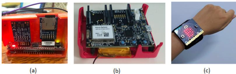
Figure 6.2: A-WEAR bracelets Fig.(a) shows First version Fig.(b) shows second version and Fig.(c) shows Final version of bracelet
