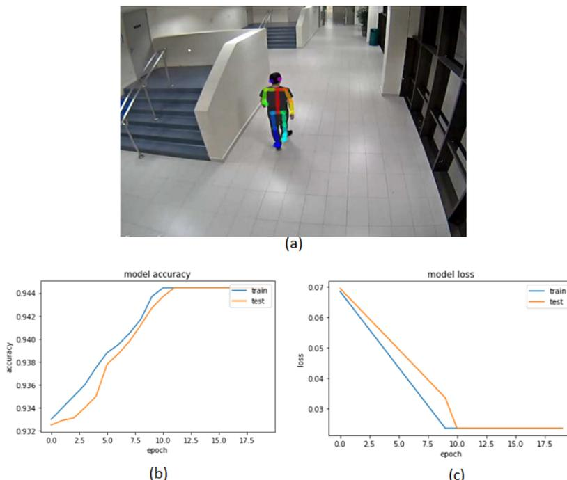
Figure 4.3: Fig (a) shows Skeleton detection from 2D image, Fig (b) explains accuracy of the proposed model during training and testing, Fig (c) illustrates the loss of the proposed model during training and testing
