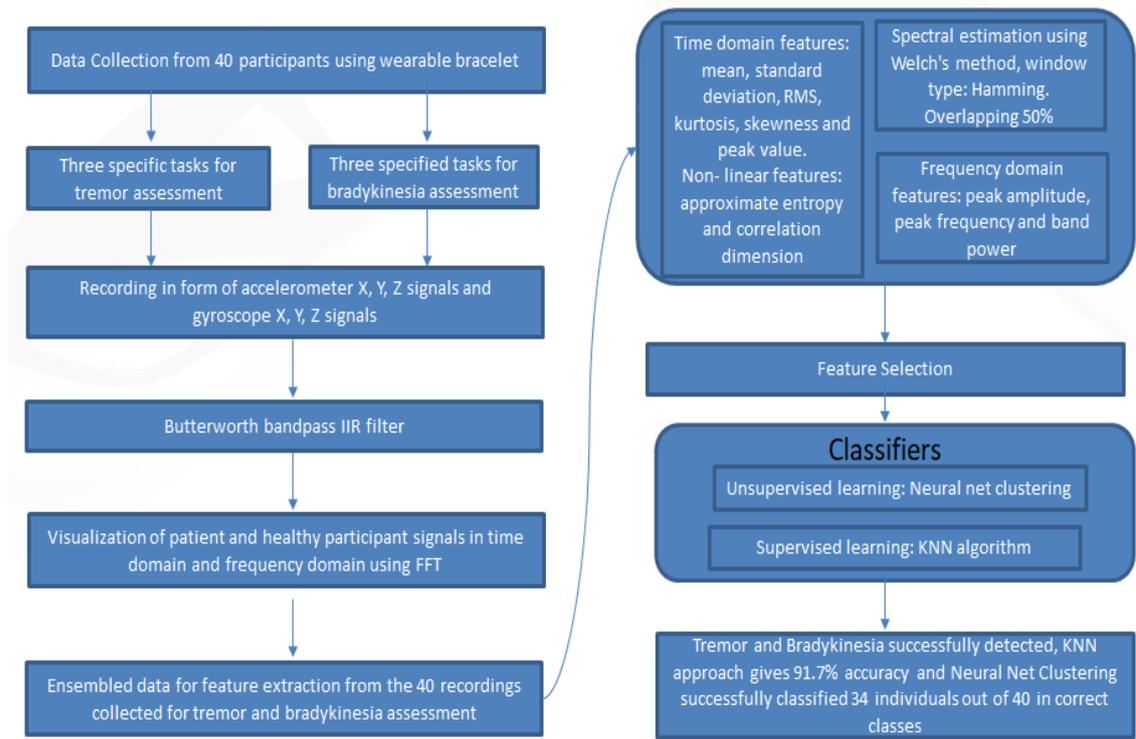
Figure 3.2: Figure illustration of the pipeline for detection of tremor and bradykinesia
