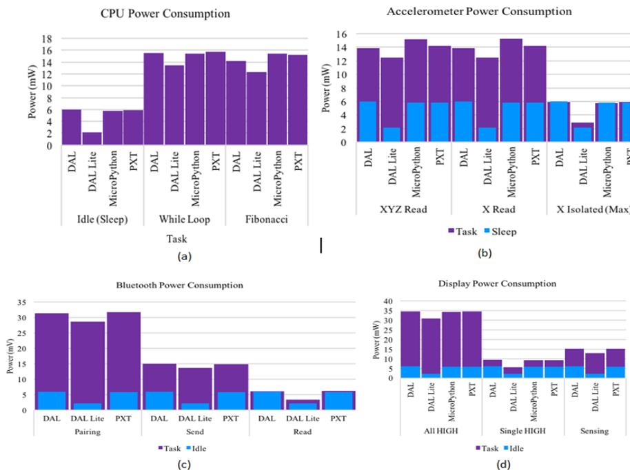
Figure 6.3: Power consumption of CPU, BLE, Matrix Lex and Accelerometer
