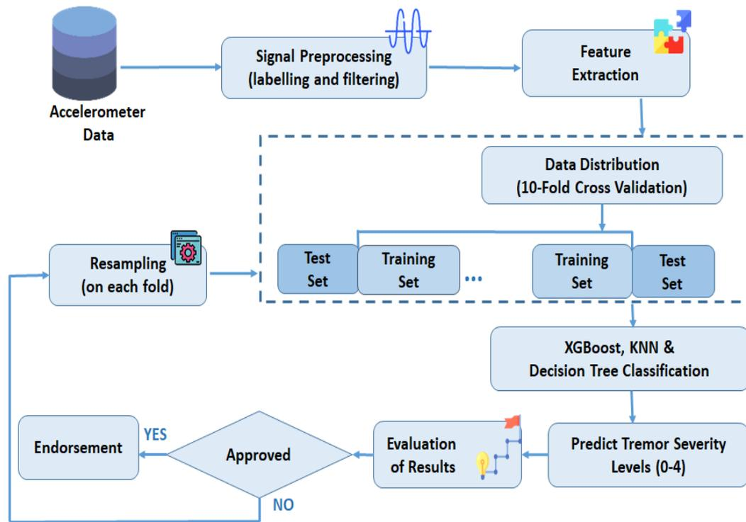
Figure 5.5: The proposed framework for tremor severity classification.
