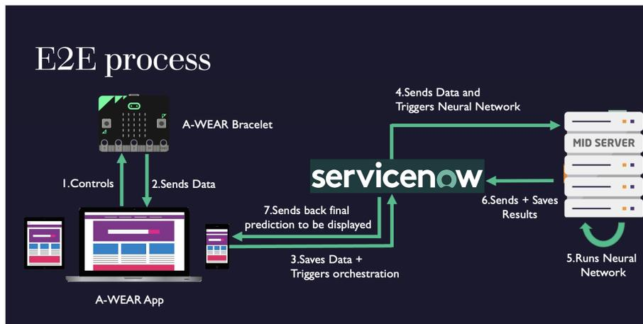
Figure 6.4: End to End process flow between A-WEAR Bracelet (micro:bit controller), A-WEAR Application (ServiceNow UI Component), and MID Server which runs the DL
