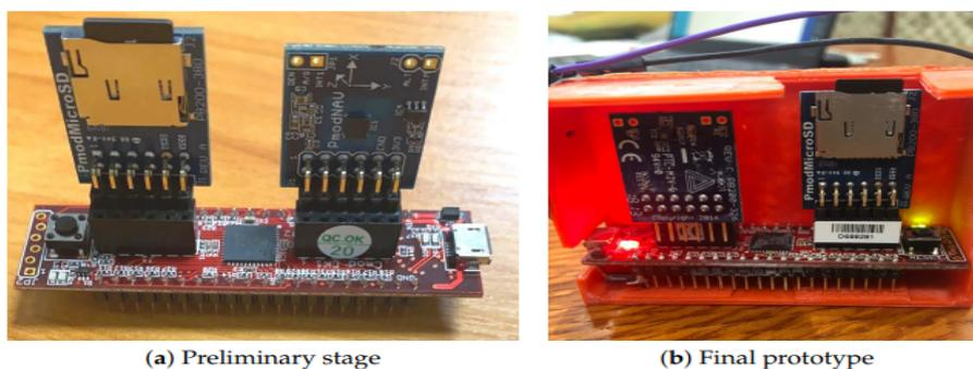
Figure 3.1: (a) Preliminary stage design of bracelet; (b) shows final prototype of A-WEAR bracelet
