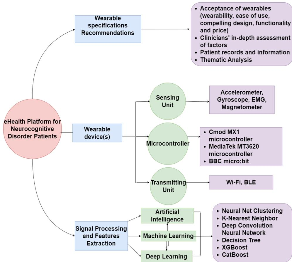
Figure 1.1: Schematic Representation of framework developed in this thesis.
