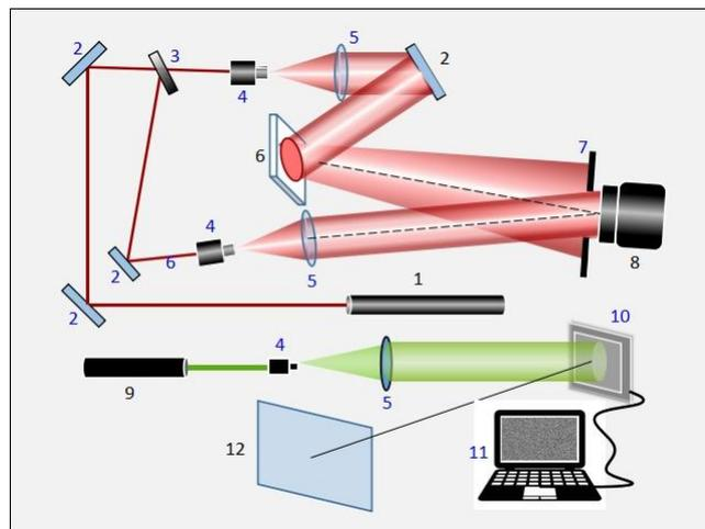
**Fig. 5.3** Schematic of the hybrid real-time holographic acquisition and reconstruction set-up: (1) He-Ne laser; (2) mirrors; (3) variable beam splitter; (4) spatial filters; (5) converging lenses for collimation; (6) diffuse object; (7) diaphragm; (8) CCD digital camera; (9) Yag:Nd laser in continuous mode (532 nm); (10) SLM LCoS HoloEye HEO 1080; (11) laptop; (12) reconstructed image projection screen.
