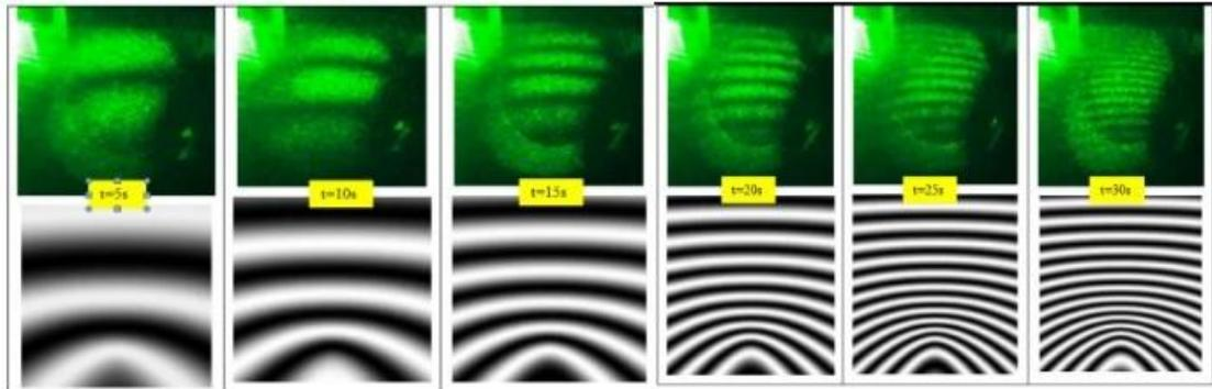
**Fig. 6.8** – Two sequences of six reconstructed images selected from the dynamic interferograms characterizing the evaporation of the water drop, experimentally (green light) and in numerical simulation (black and white).
