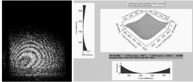
**Fig. 6.2** Interference fringes generated by the optical path difference induced by the presence of water in a quartz cuvette, the first holographic frame acquired being that of the empty cuvette (a); a distribution of optical path difference illustrated by fringes (b).
