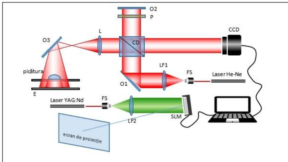
**Fig. 6.9** Schematic of the real-time DHI experimental set-up for monitoring the evaporation of a water drop from a horizontal surface: polarized He-Ne laser (633 nm); frequency-doubled Nd:YAG laser (532 nm); FS - spatial filter; L, LC1, LC2 - collimating lenses; O1, O2, O3 - plane mirrors; P - polarizer (used as an attenuator); CD - dividing cube; E - matte white screen.
