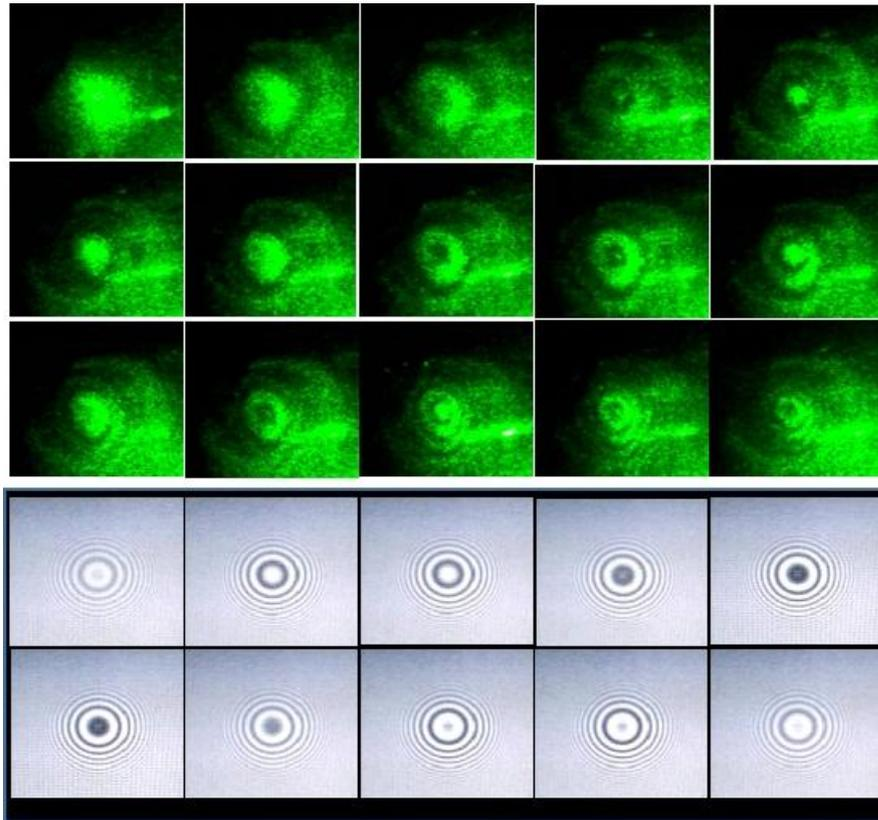
*Fig. 6.11* Successive frames from a dynamic sequence of interferograms obtained by real-time holographic interferometry (green light) and white light interferometry generated by the evaporation of a water droplet from a horizontal surface.
