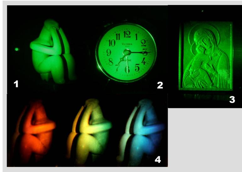
*Fig. 3.6 Photographs of images reconstructed by classical Fresnel holography (1, 2, 3), image type (4, the three images are taken from different angles to observe the entire color spectrum) made on holographic plates in the Optical Spectroscopy and Laser Laboratory of the INFLPR*
