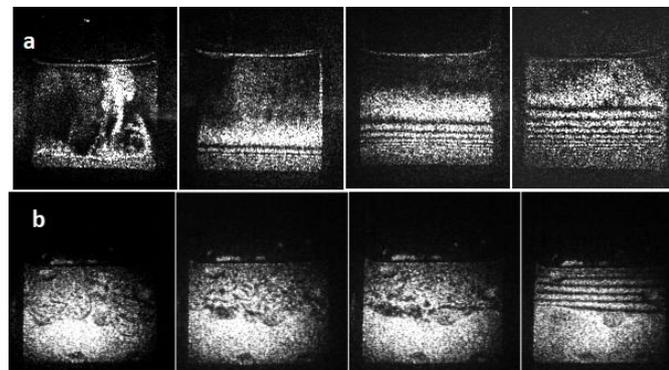
**Fig. 6.4** The sequence of 4 images reconstructed from interferograms recorded in real time (22 fps) in which a dissolution process of two liquids is presented: a) saturated saline solution in water (in the first image you can see the convection generated by a drop of saturated solution of NaCl in water); b) ethanol in water
