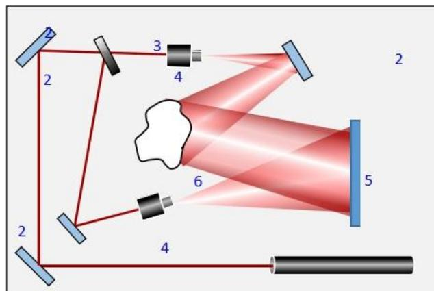
**Fig. 3.5** Scheme of an experimental Fresnel holography set-up used in classic holographic recordings on emulsion plates: He-Ne Laser ( $\lambda = 632.8 \text{ nm}$ ) (1); mirrors (2); variable beam splitter (3); spatial filters (4); holographic plate - hologram (5); the object (6)
