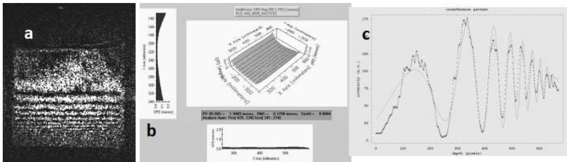
**Fig. 6.5** Reconstruction of a holographic interferogram generated by a quartz vat filled with water in which NaCl was dissolved. (a); Refractive index distribution correlated with OPD distribution generated with IntelliWave (b); Intensity distribution as a function of depth (c).
