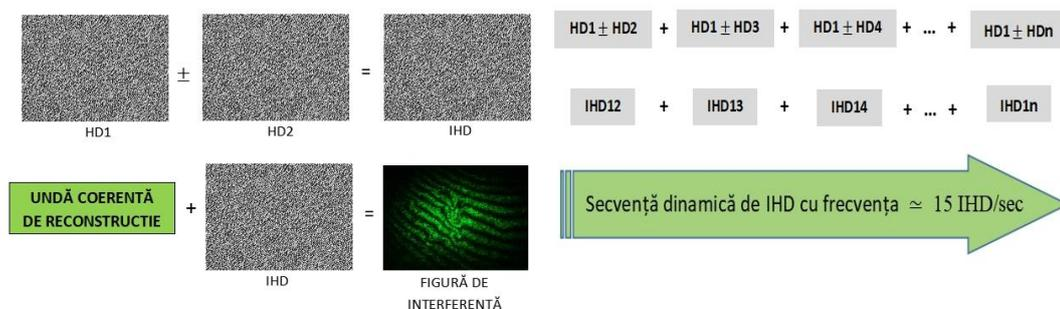
*Fig. 4.1 Schematic representation of digital formation and reconstruction processes in digital holographic interferometry applications.*
