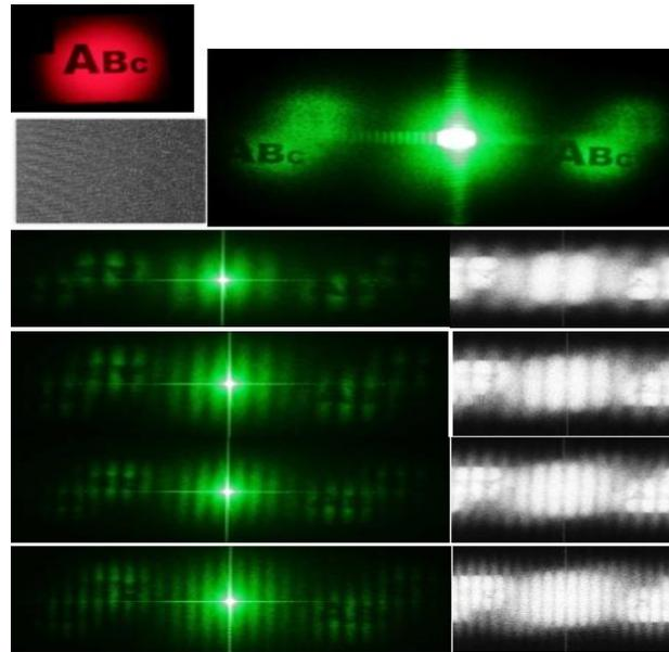
**Fig. 5.5** Real-time sequence of four holographic interferograms corresponding to lateral displacements from a sequence of frames digitally recorded and reconstructed with the HoloEye HEO 1080 spatial phase modulator: a) diffuse object illuminated with coherent wave; b) digitally recorded amplitude hologram c) reconstruction wave diffraction on the SLM displaying the phase hologram; d) sequence of holographic interferograms e) sequence of numerically calculated holographic interferograms
