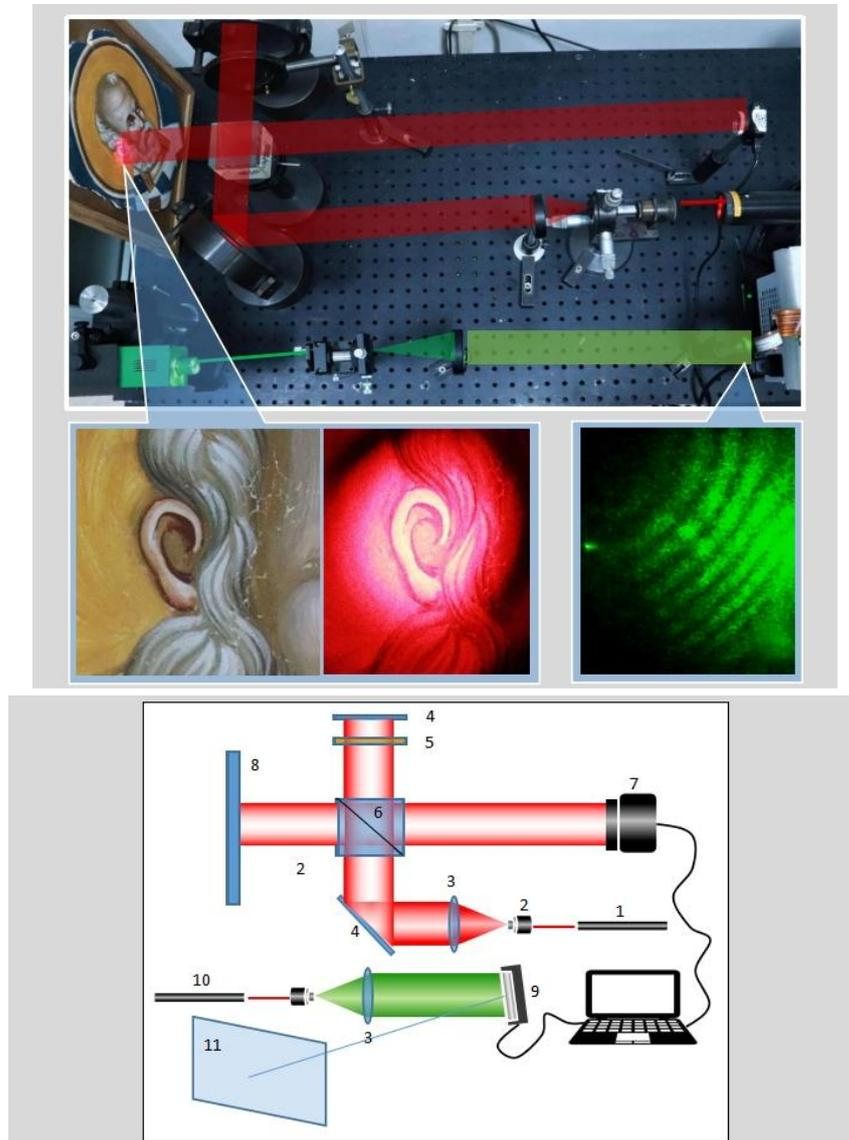
**Fig. 5.8** Laboratory image and scheme of the experimental setup of DHI in Michelson configuration, used in the study of structural defects of a surface painted in the "fresco" technique (1) linearly polarized He-Ne laser; (2) spatial filters; (3) collimating lenses; (4) plane mirrors; (5) polarizer; (6) dividing cube; (7) CCD camera; (8) object; (9) HoloEye HEO 1080 digital spatial phase modulator; (10) YAG:Nd laser in continuous mode 532 nm; (11) interference figure projection screen.
