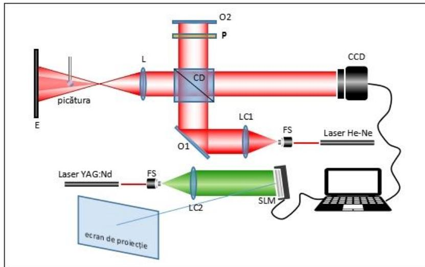
**Fig. 6.7** Real-time DHI setup for monitoring the evaporation of the water droplet in suspension: polarized He-Ne laser (633 nm); frequency-doubled Nd:YAG laser (532 nm); FS - spatial filter; LC1, LC2 - collimating lenses; O1, O2 - plane mirrors; P - polarizer (used as an attenuator); CD - dividing cube; E - matte white screen.
