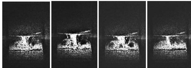
**Fig. 6.3** Sequence of 4 images reconstructed at one second intervals of the convection process observed in real time by DHI
