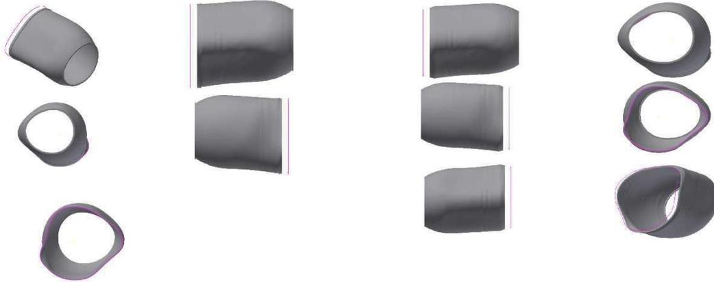
Fig. 5.45. Cup components for epoxy resin and fiberglass mat filling variant - First component (interior)
