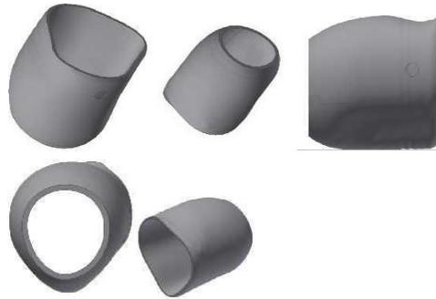
Fig. 5.44. The constructive version of the cup for filling with epoxy resin
