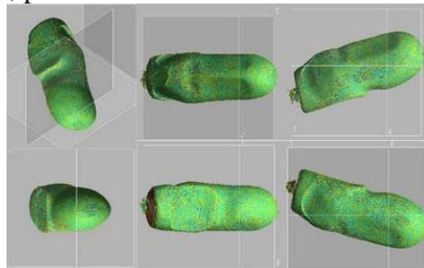
*Fig. 3.5. The abutment digitized by photogrammetry. Different views from the \*.STL file.*
