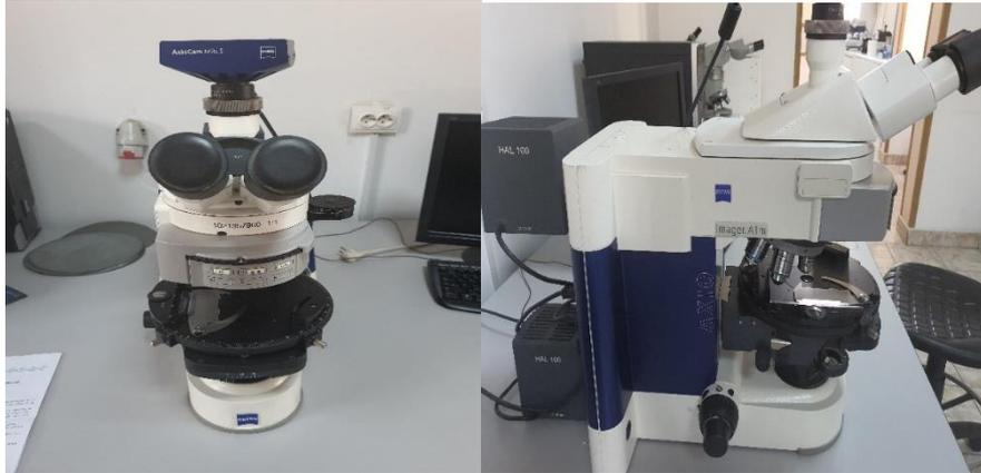
**Fig.6.20** Optical microscopy apparatus Carl Zeiss AXIO IMAGER A1m
