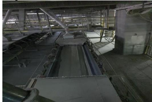
**Fig.6.92 b) Left conveyor belt for fine cement**
