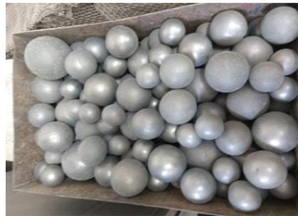
**Fig.6.29** Grinding balls of different sizes, [19]
