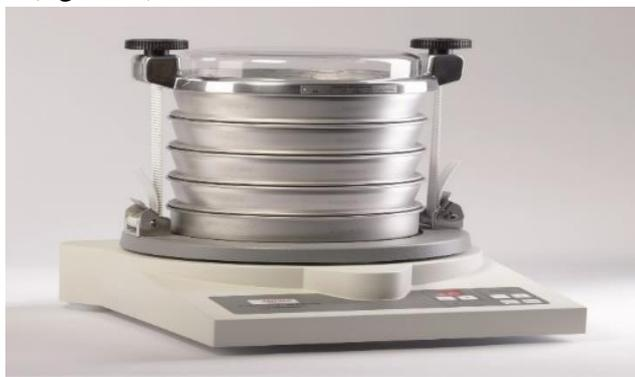
**Fig.6.27** Classifier with site Analysette 3 Spartan, [162]
