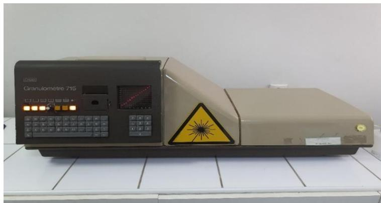
**Fig.6.19** CILAS - Delcita 715 laser granulometric analysis device
