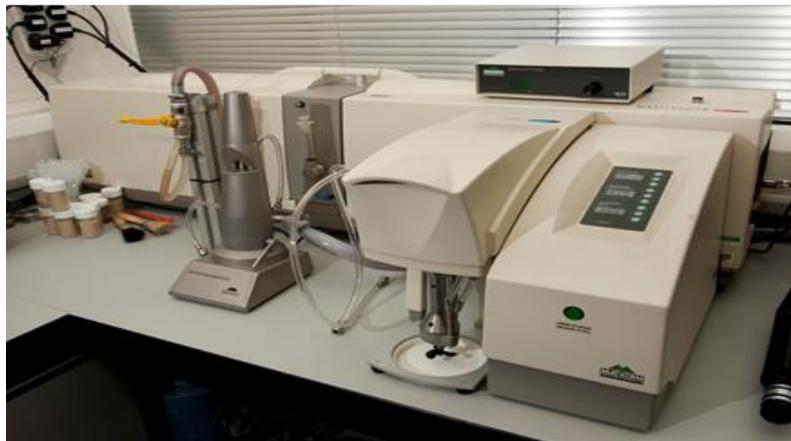
**Fig.6.18** Mastersizer 2000E laser granulometric analysis device, [18,152]
