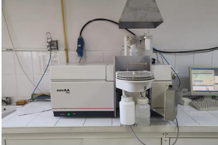
**Fig.6.17** NovAA 400 clinker chemical analysis apparatus
