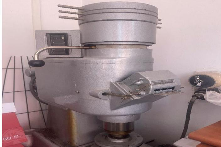
**Fig.6.24** Zeisel Apparatus for grindability determination
