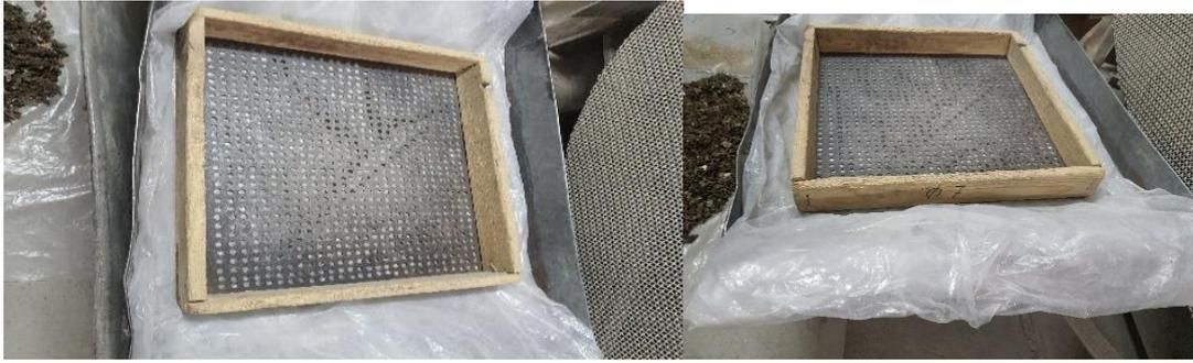
**Fig.6.7** Grinding sieve of diameter  $\varnothing=7$  mm
