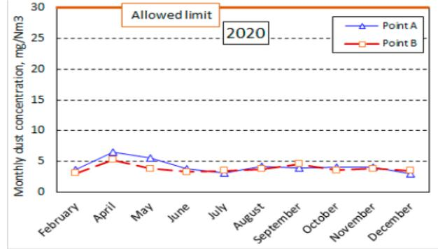
Fig.6.96 b) The distribution of dust emissions at the Cement Mill Separator No. 1 from the monitored cement plant, [16]
