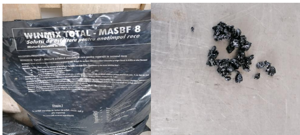
Fig. 5.8. Medium grain material for repairs
