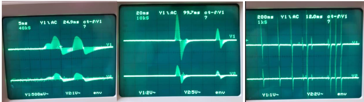
a) b) c) Fig.3.3. Voltage recording at the passage of: a-car, b-truck, c-trailer
