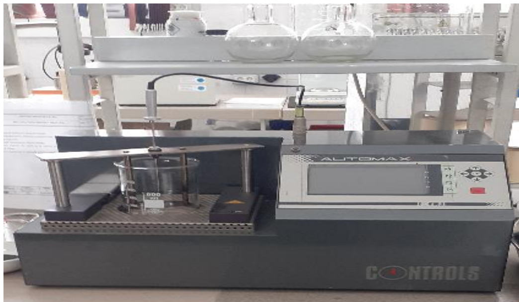
Fig. 5.11. “Ring and Ball Tester” automatic equipment
