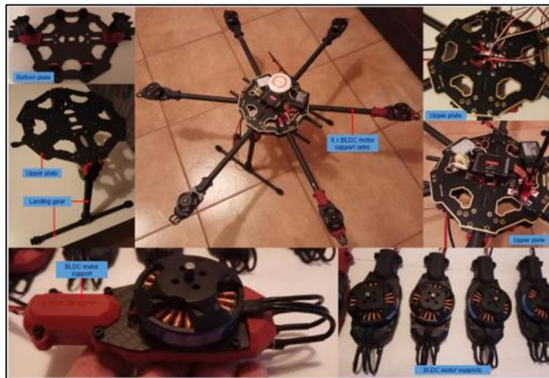
Fig. 4.4 Hexacopter structure, by component
