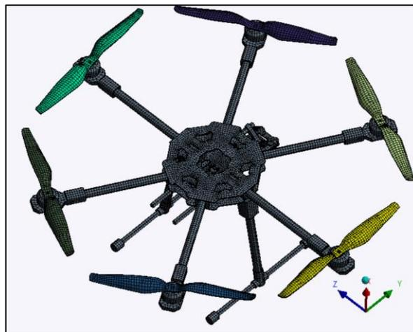
Fig. 5.9. Discretization for structural analysis
