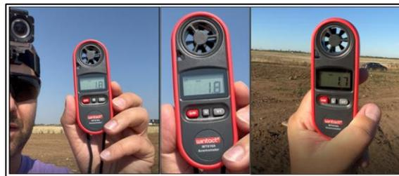
Fig. 4.14 Measuring wind speed with an anemometer
