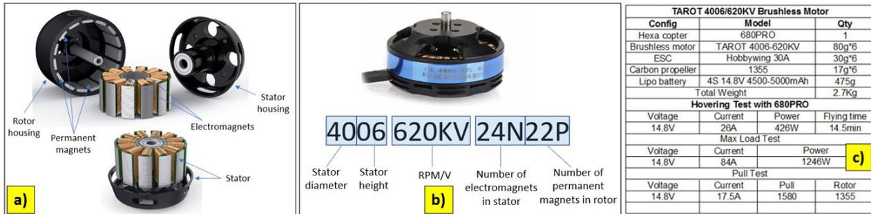
Fig. 3.3 a) Brushless DC electric motor with external rotor (outrunner); b) Tarot 4006/620KV 24N22P motor with which HUT is equipped [28]; c) Tarot 4006/620KV 24N22P motor performance [28].
