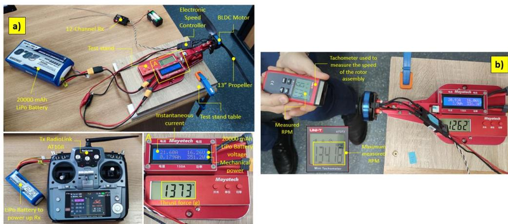
Fig. 3.16 a) Propulsion system efficiency test stand configuration; b) Measurement of rotor speed
