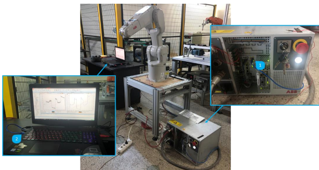
Fig. 3.9. The experimental setup consisting of an articulated robot IRB 1200, featuring the connection between the IRC5 controller (1) and the laptop running RobotStudio (2)
