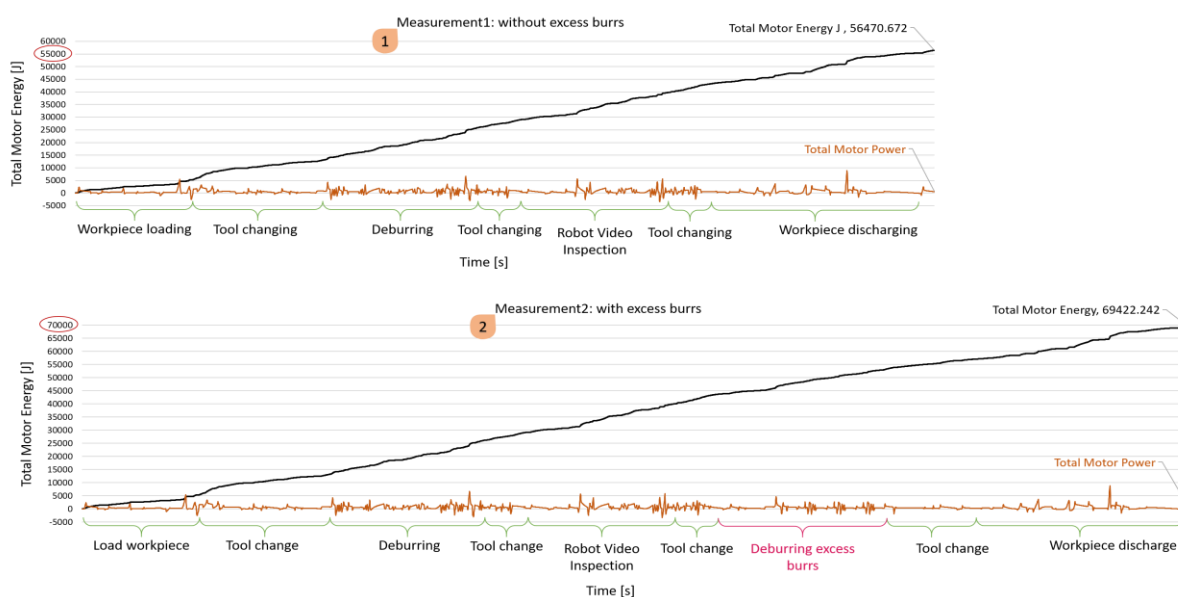
Fig. 4.6. Total energy (black) and total power (orange) of the robot during a deburring work cycle with no remaining burrs (1) and with remaining burrs (2).
