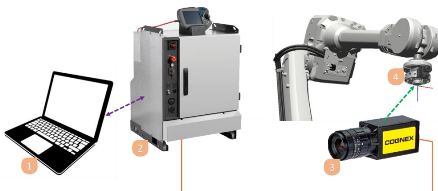
Fig. 4.5. Vision system equipment: PC running ABB RobotStudio (1), robot controller (2), Cognex 8400 camera (3), the ATC system (4).
