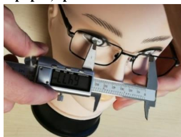
Fig.6.6. Caliper measurement of mannquin pupillary distance (64.77 mm) [67]
