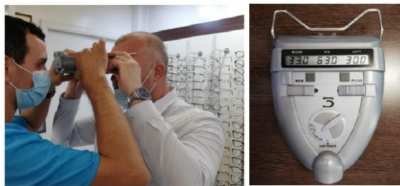
Fig.6.26 Interpupillary distance measured with the electronic pupildimeter (George Baboianu)
