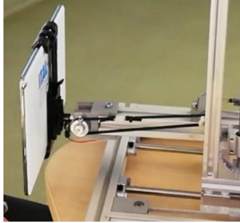
Fig.6.1. The tablet mounted in the special support, attached to the arm of the device
