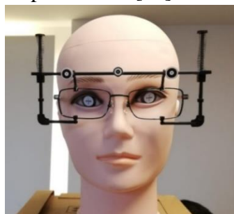
Fig.6.5. Mannequin with pupils, spectacle frame and frame with markers [67]
