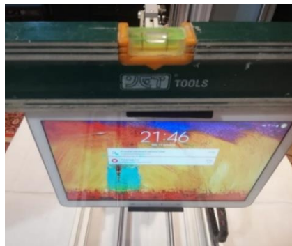
Fig.6.2. Horizontality verification of the tablet
