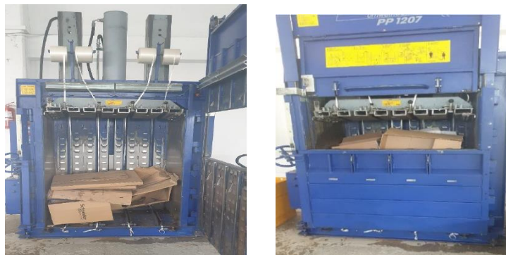
Fig.6.17. Aspects during the experimental determination when compacting cardboards
