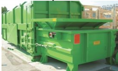
Fig. 3.8. Compaction system by traslation, with fixed location, for waste from building materials and removable container
