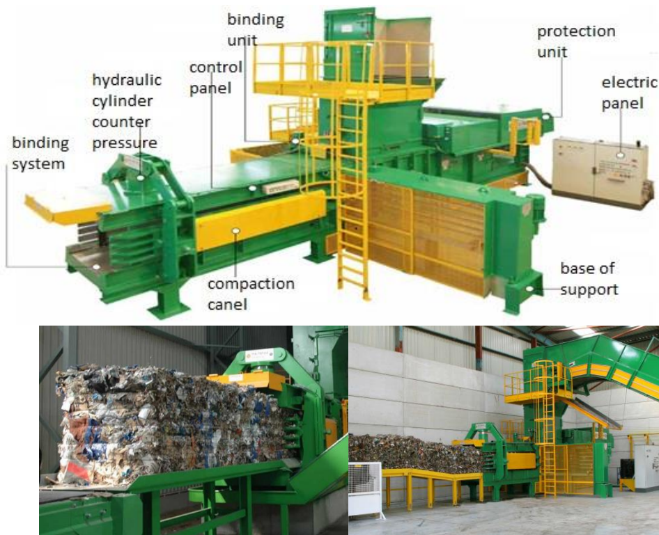
Fig. 3.3. Baling- packing installation
