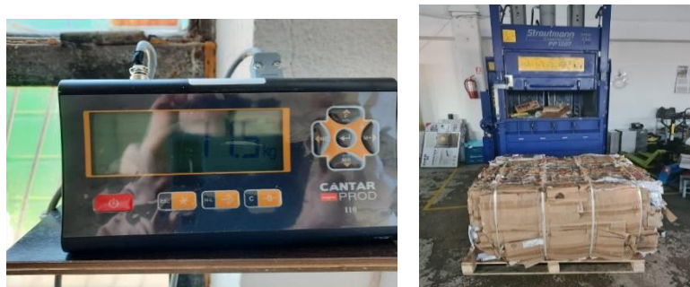
Fig.6.16. Test press and bound bale obtained after compaction/baling
