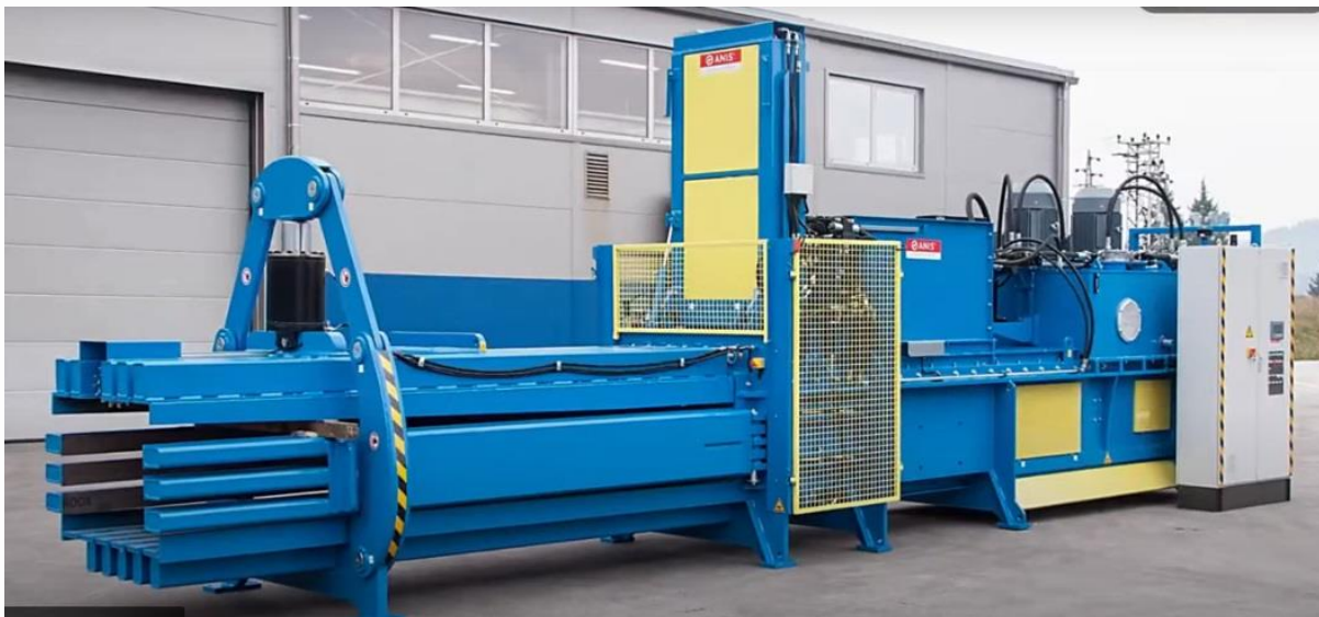
Fig.6.25. Overview of the horizontal press for bales of recyclable waste
