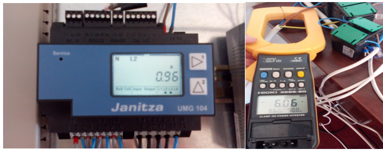
Indication of the numerical counter I_{2s} = 0,96A Current I_2 measured multimeter = 6,06A
