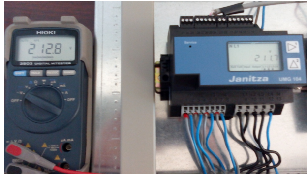
Measurement of voltage phase U_{IN} : measured U_{IN} = 211,7 \text{ V} ; standard U_{eIN} = 212,8 \text{ V}
