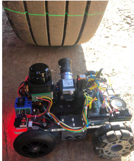
Fig. 5.12 Example of the optimal position for the camera and laser beam.
