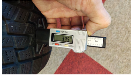
Fig. 5.20 Manual measurement of tire tread with a digital caliper.
