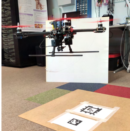
Fig. 3.8 The drone flying in our office. The image was taken after the target was acquired and the camera was automatically oriented towards the target.
