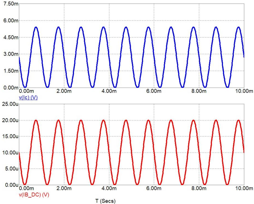
Fig. 4.3.6. Transient analysis for a BC817 transistor [circuit made in SPICE, BF=270, IKF=1800mA].
