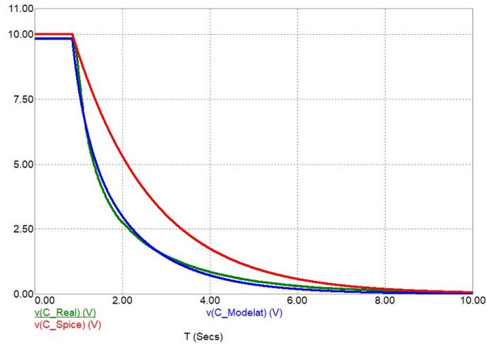
Fig. 3.1.6. Time variation of the discharge of a real capacitor compared to a model modeled in SPICE and a SPICE model.
