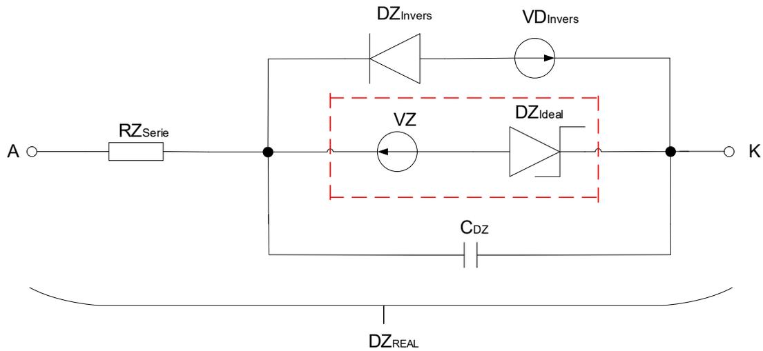
Fig. 4.2.1. The equivalent circuit of a real stabilizer diode.
