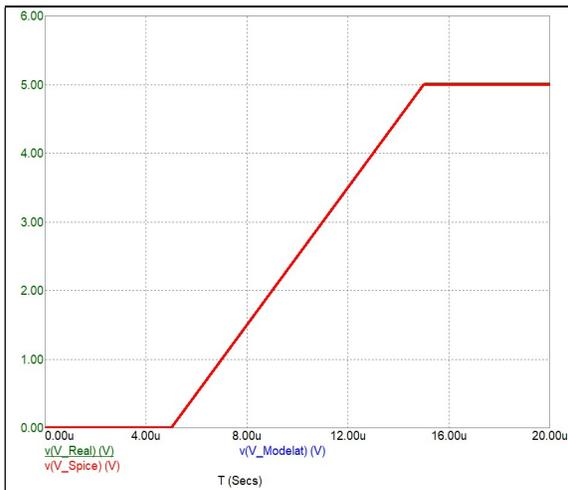
Fig. 3.3.5. Time variation of the voltage drop across a real resistor compared to a nonlinear model modeled in SPICE and a SPICE model to a ramping increase in supply voltage.
