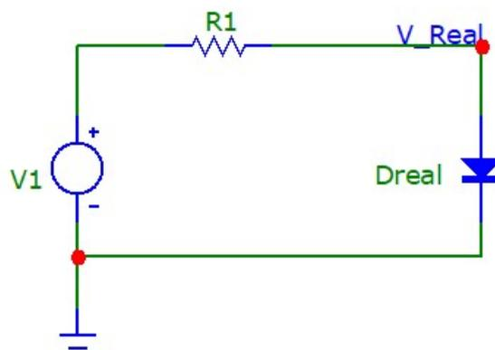
Fig. 4.1.3. Voltage drop across a real diode – practical circuit.
