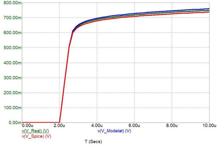
Fig. 4.1.6. Voltage drop across a real diode compared to a SPICE modeled nonlinear diode and a SPICE model diode (I=10mA).
