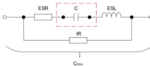
Fig. 3.1.1. The equivalent circuit of a real capacitor.
