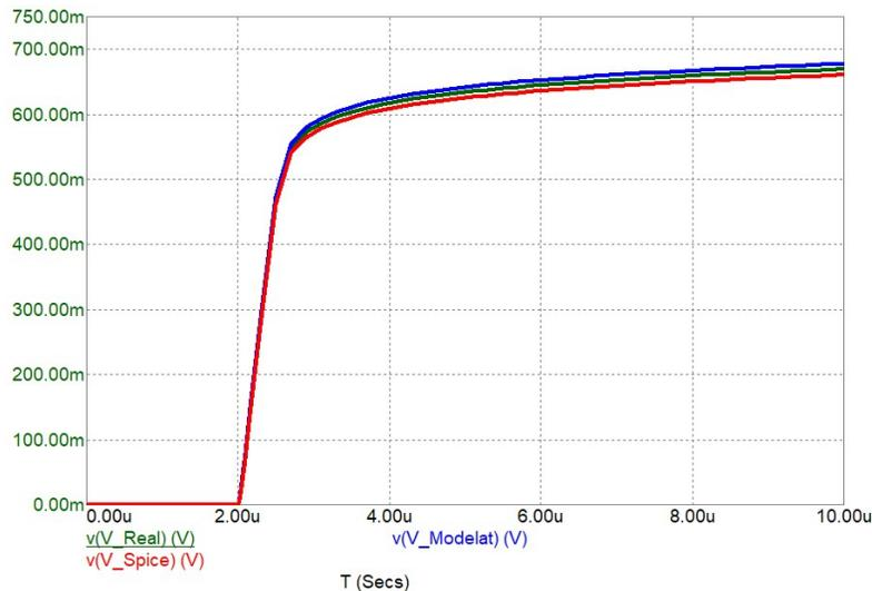
Fig. 4.1.5. Voltage drop across a real diode compared to a SPICE modeled nonlinear diode and a SPICE model diode.
