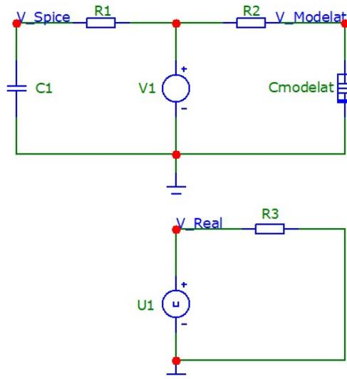
Fig. 3.1.4. Charge and discharge circuit of a capacitor made in SPICE.
