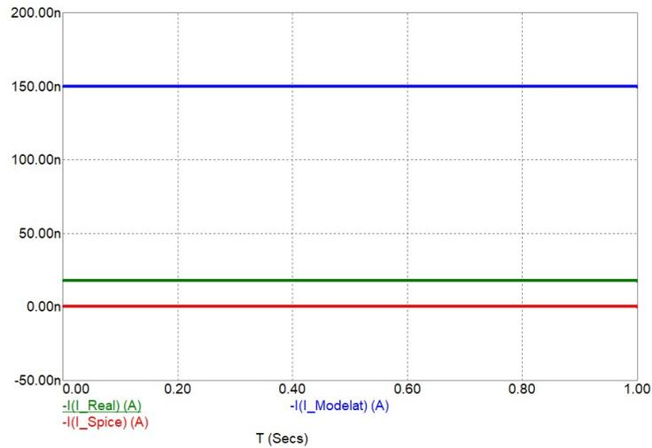
Fig. 4.1.10. Current through a real diode compared to a SPICE modeled diode and a SPICE model diode.
