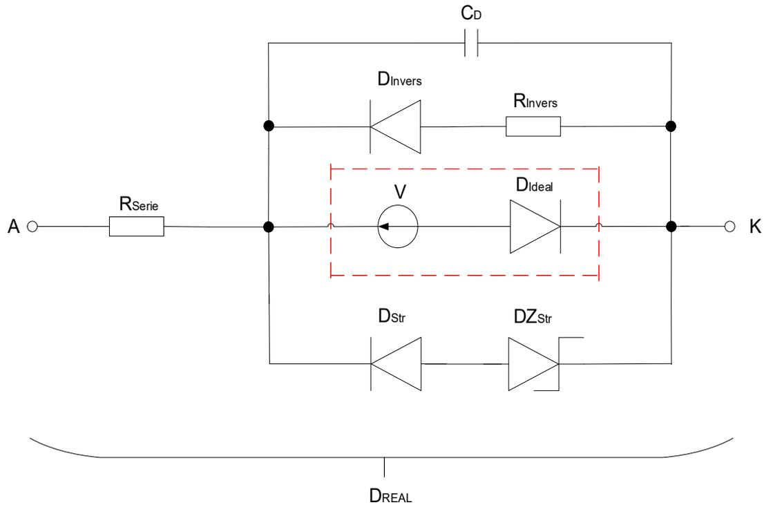
Fig. 4.1.1. The equivalent circuit of a real rectifier diode.
