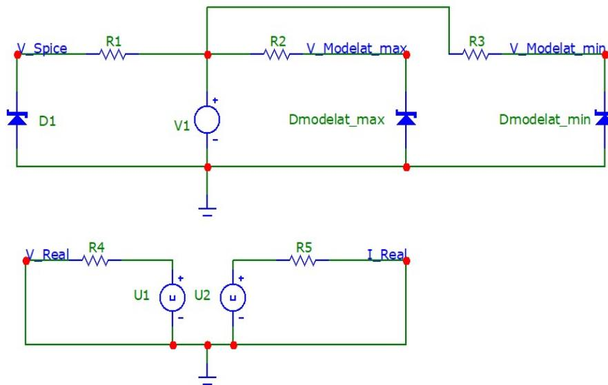
Fig. 4.2.4. Voltage drop across a stabilizer diode (modeled in SPICE, SPICE, Real) – circuit made in SPICE.
