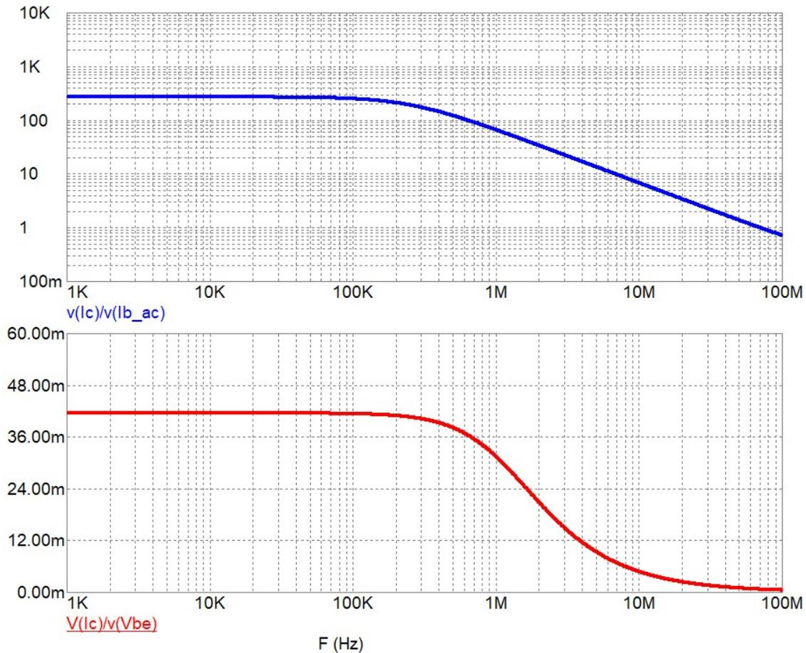
Fig. 4.3.9. AC analysis for a BC817 transistor to determine  $h_{FE}$ ,  $G_m$  [circuit made in SPICE,  $BF=270$ ,  $IKF=1800mA$ ,  $R_{BB}=1400\Omega$ ,  $R_{EE}=10\Omega$ ,  $TF=467ps$ ].
