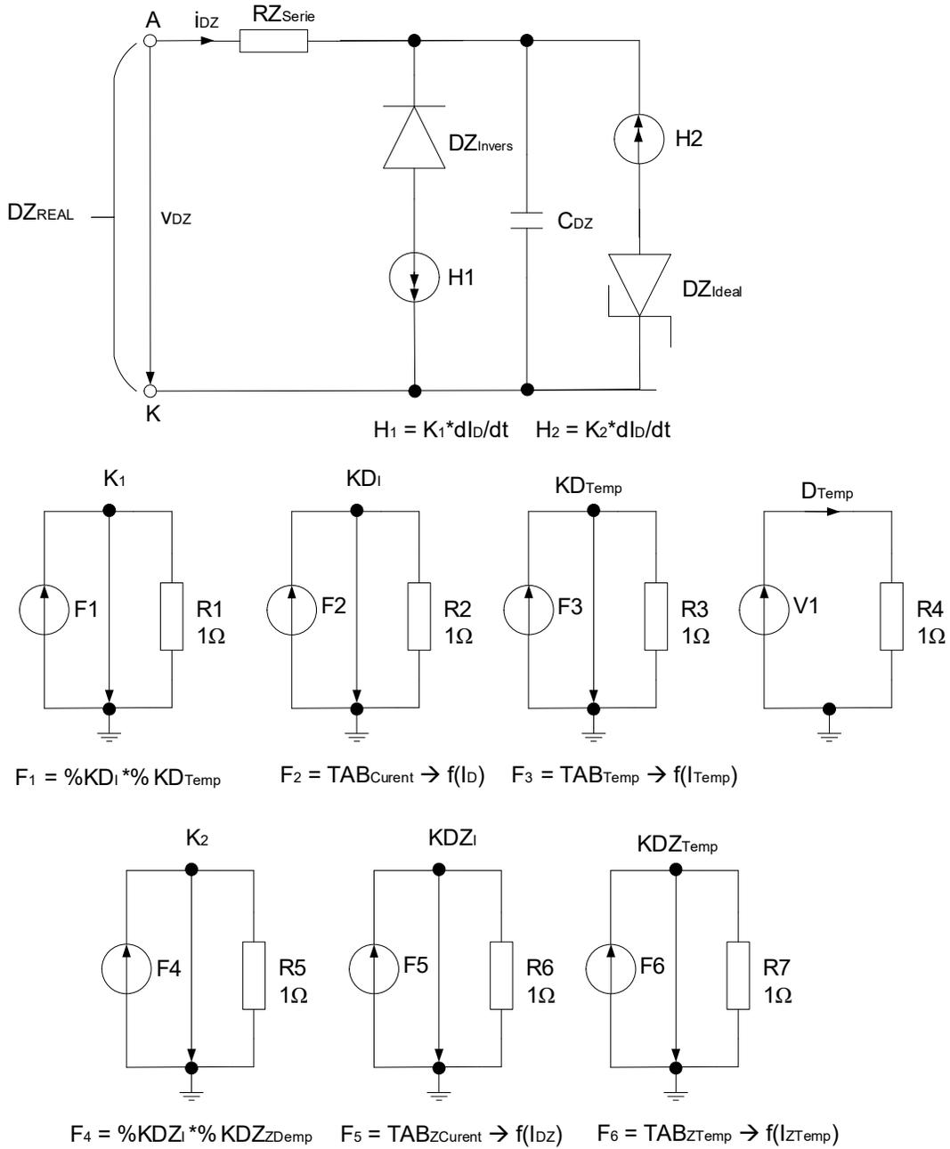
Fig. 4.2.2. SPICE model of a real stabilizer diode.
