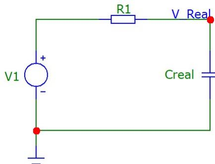
Fig. 3.1.3. Charging and discharging circuit of a practically made capacitor.
