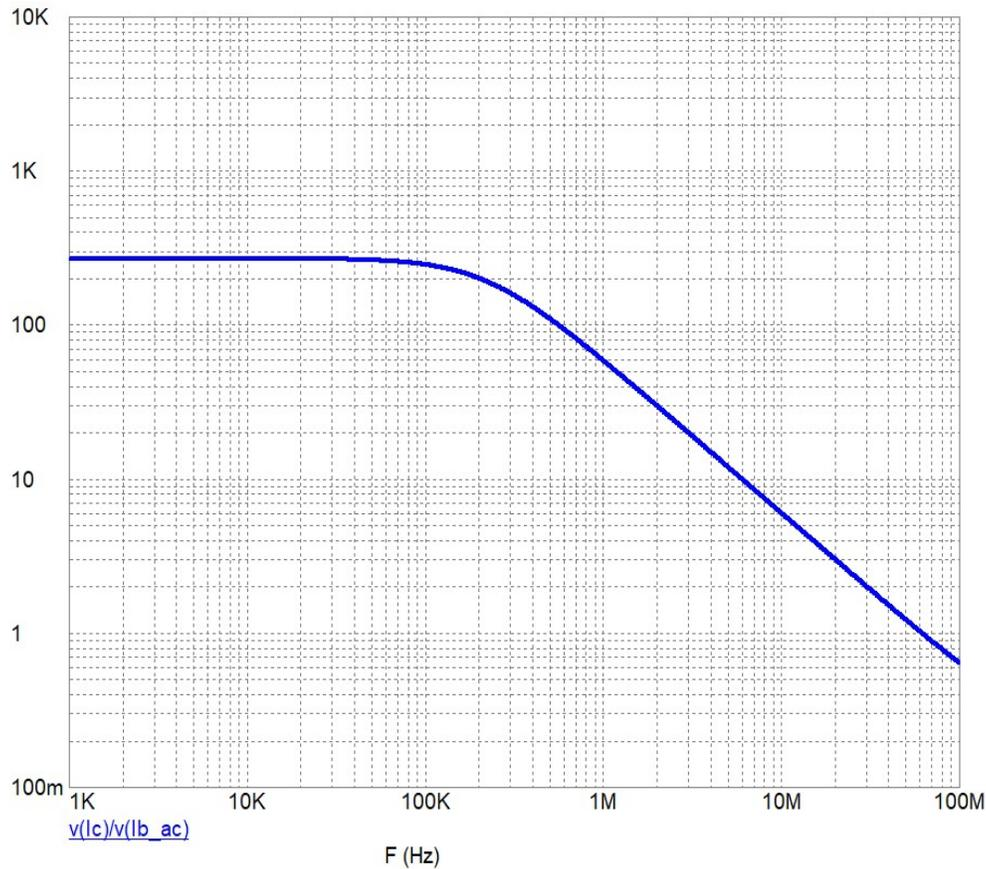
Fig. 4.3.7. AC analysis for a BC817 transistor [circuit made in SPICE,  $BF=270$ ,  $IKF=1800\text{mA}$ ].
