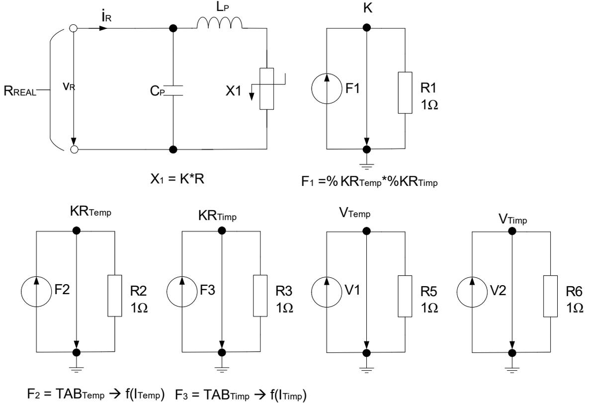
Fig. 3.3.2. SPICE model of a real non-linear resistor.
