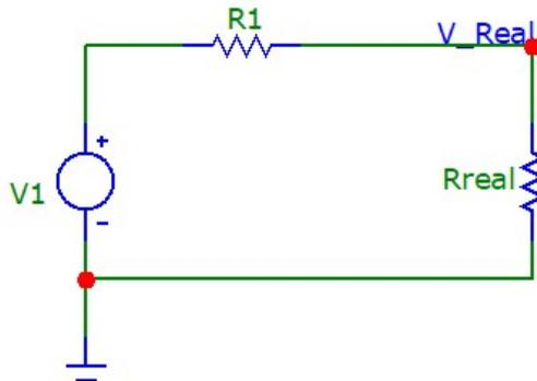
Fig. 3.3.3. Practically made resistive divider.
