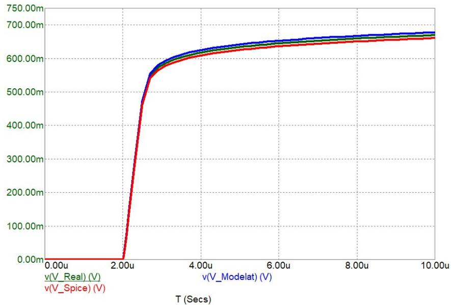
Fig. 4.2.8. Voltage drop across a real Zener diode compared to a SPICE modeled Zener diode and a SPICE model Zener diode.
