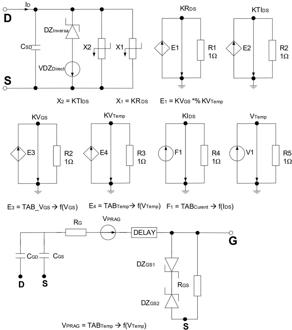
Fig. 4.4.2. SPICE model of a 'n' channel MOSFET transistor.
