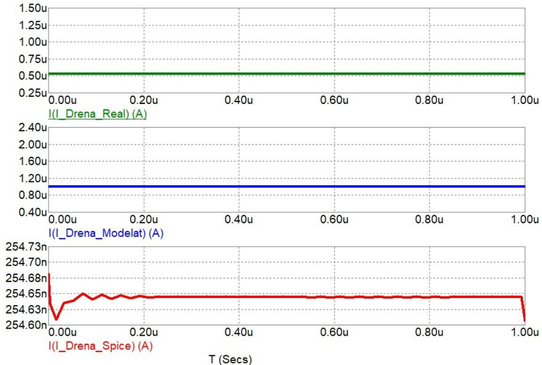
Fig. 4.4.6. Drain-source leakage current of a real MOS-FET compared to a SPICE-modeled MOS-FET and a SPICE MOS-FET.
