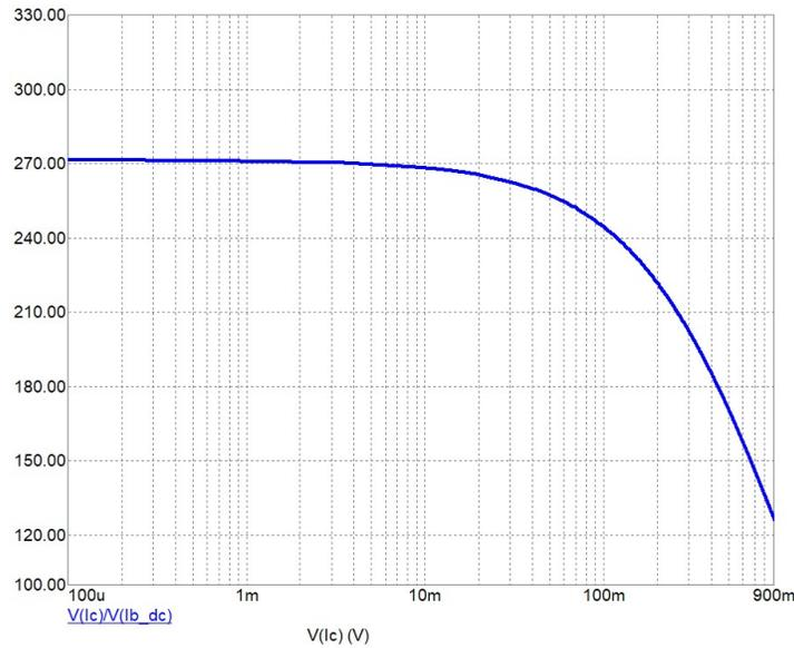
Fig. 4.3.4. DC analysis of  $H_{FE}$  amplification factor as a function of collector current for a BC817 transistor [circuit made in SPICE, BF=270, IKF=900mA].
