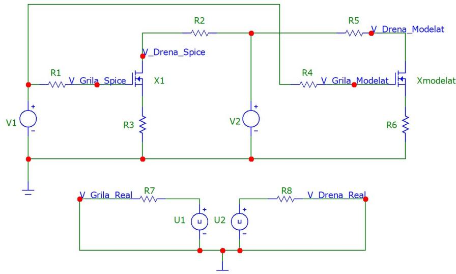
Fig. 4.4.4. Circuit made in SPICE for the study of the "n" channel MOS-FET transistor (IRFH3707) (Modeled, SPICE, Real).
