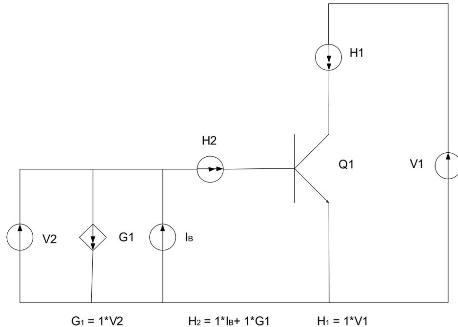
Fig. 4.3.1. Architecture of a circuit that helps to check the parameters of an NPN bipolar transistor.
