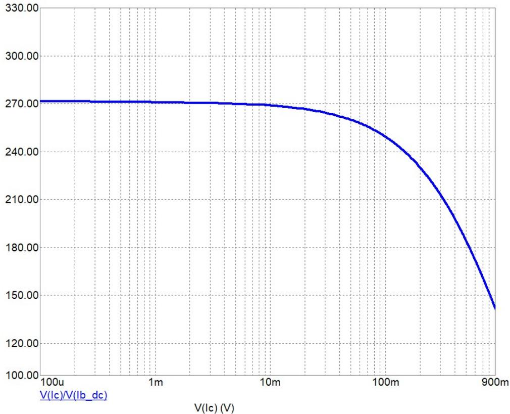
Fig. 4.3.5. DC analysis of HFE amplification factor as a function of collector current for a BC817 transistor [circuit made in SPICE,  $BF=270$ ,  $IKF=1800mA$ ].
