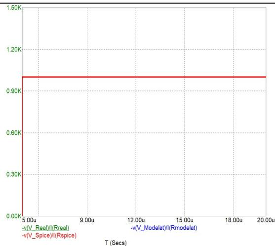
Fig. 3.3.6. The resistance value of a real resistor compared to a non-linear model modeled in SPICE and a SPICE model to a ramping increase in supply voltage.
