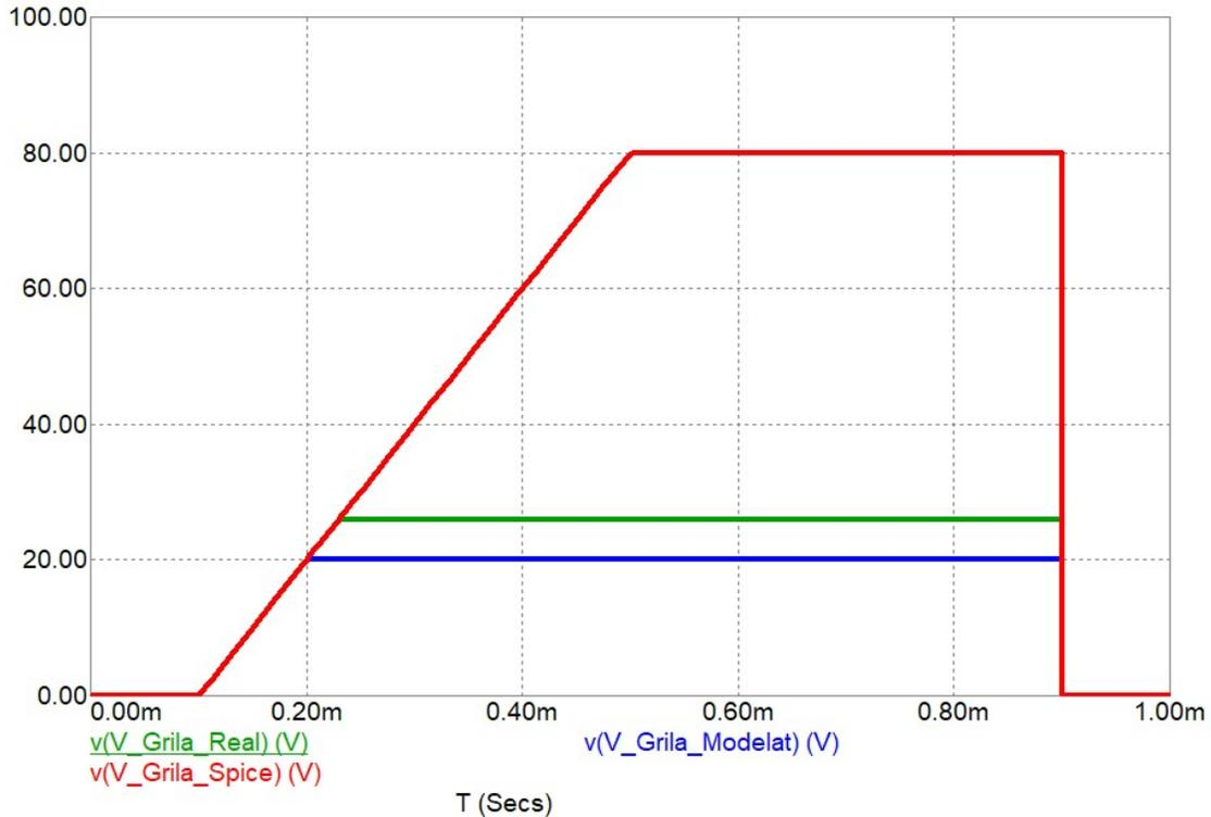
Fig. 4.4.8. Grid-source breakdown voltage of a real MOS-FET compared to a SPICE-modeled MOS-FET and a SPICE MOS-FET.
