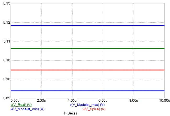
Fig. 4.2.5. Voltage drop across a real Zener diode compared to a SPICE-modeled nonlinear Zener diode and a SPICE-modeled Zener diode.
