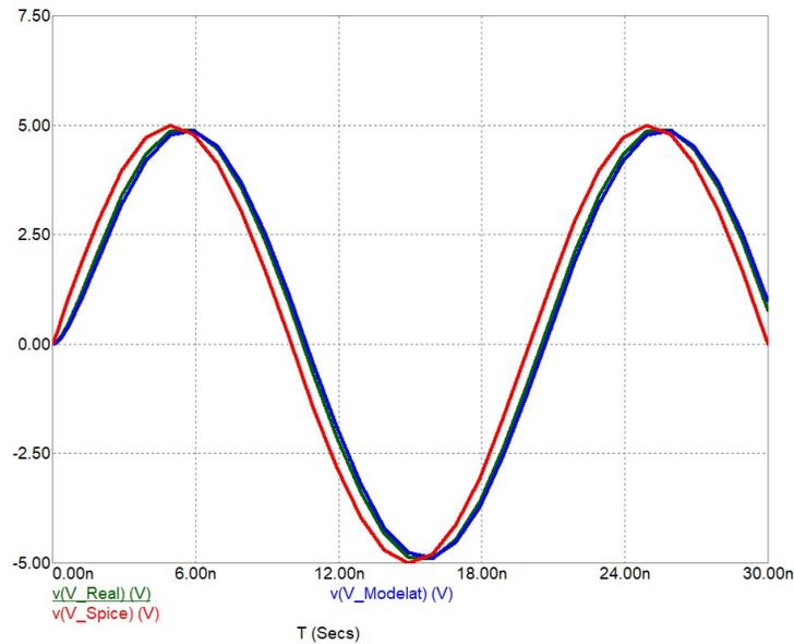
Fig. 3.3.7. Time variation of the voltage drop across a real resistor compared to a nonlinear model modeled in SPICE and a SPICE model at a frequency of 50MHz.
