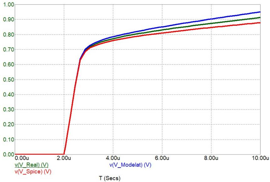
Fig. 4.1.7. Voltage drop across a real diode compared to a SPICE modeled diode and a SPICE model diode ( $I=100\text{mA}$ ).
