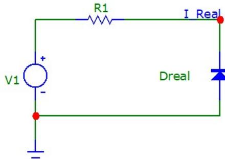
Fig. 4.1.81. Circuit to check the leakage current through a real diode - practical circuit.
