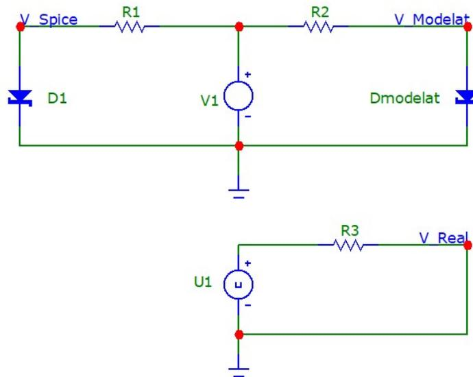
Fig. 4.2.7. Voltage drop across a stabilizer diode (modeled in SPICE, SPICE, Real) – circuit made in SPICE.
