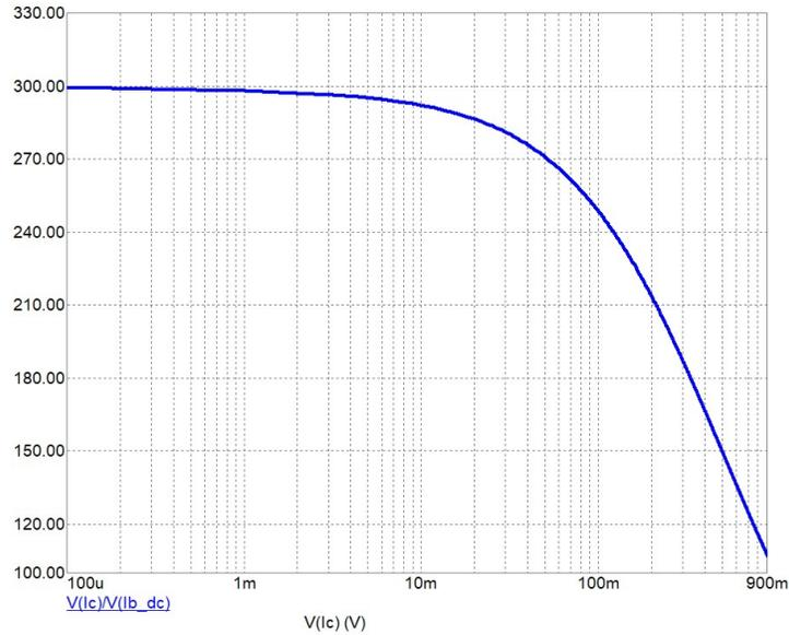
Fig. 4.3.3. DC analysis of  $H_{FE}$  gain factor as a function of collector current for a BC817 transistor [circuit simulated in SPICE].
