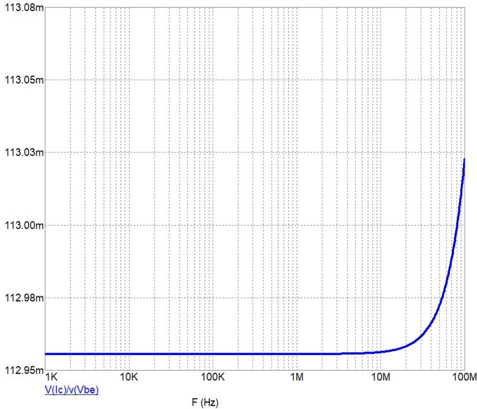
Fig. 4.3.8. AC analysis for a BC817 transistor to determine  $G_m$  [circuit made in SPICE,  $BF=270$ ,  $IKF=1800mA$ ].
