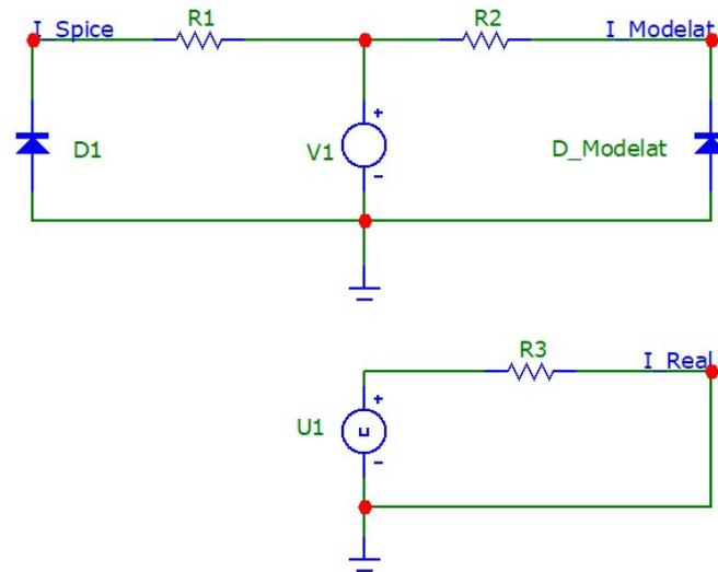
Fig. 4.1.9. Circuit to Check Current Through a Diode (Modeled in SPICE, SPICE, Real) – circuit made in SPICE.
