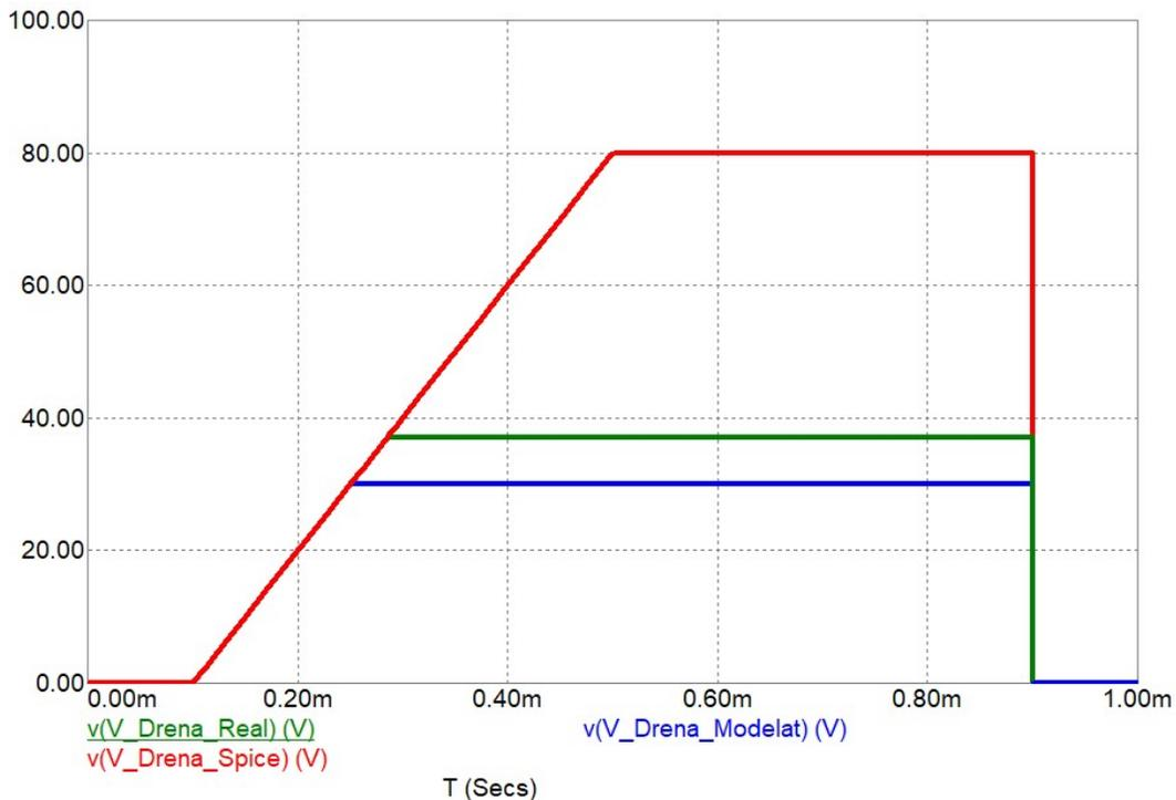
Fig. 4.4.7. Drain-source breakdown voltage of a real MOSFET compared to a SPICE-modeled MOS-FET and a SPICE MOS-FET.
