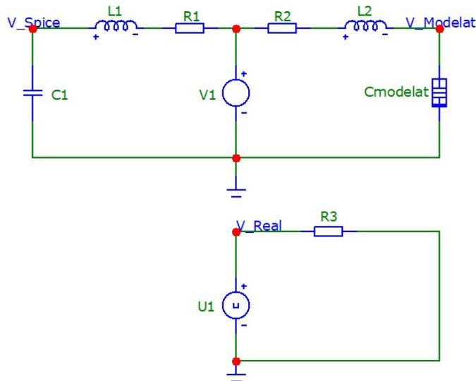
Fig. 3.1.8. Oscillating circuit made in SPICE.
