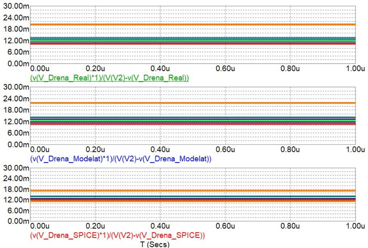
Fig. 4.4.9. Variation of drain-source resistance of a real MOS-FET compared to a SPICE-modeled MOS-FET and a SPICE MOS-FET as a function of grid-source voltage (ambient temperature is 25°C).
