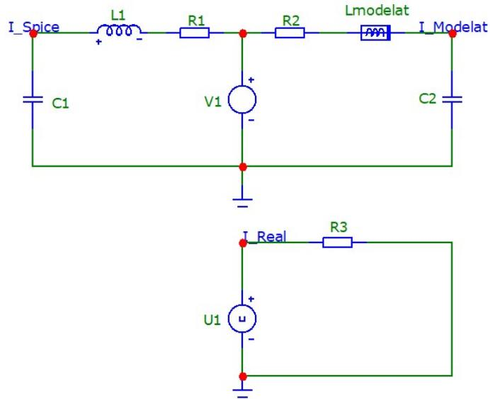
Fig. 3.2.4. Oscillating circuit made in SPICE.
