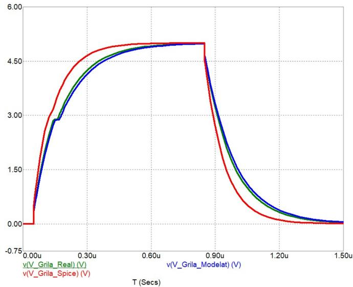
Fig. 4.4.5. Grid-source voltage of a real MOS-FET compared to a SPICE modeled MOS-FET and a SPICE-model drain to “air” MOS-FET.
