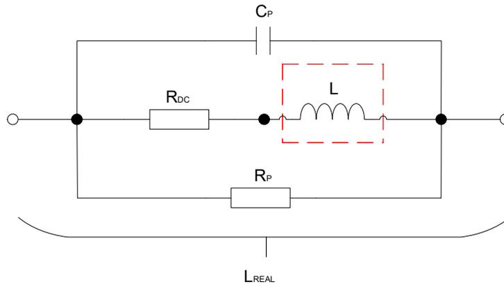
Fig. 3.2.1. The equivalent circuit of a real coil.
