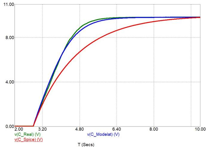
Fig. 3.1.5. Time variation of the charge of a real capacitor compared to a model modeled in SPICE and a SPICE model.
