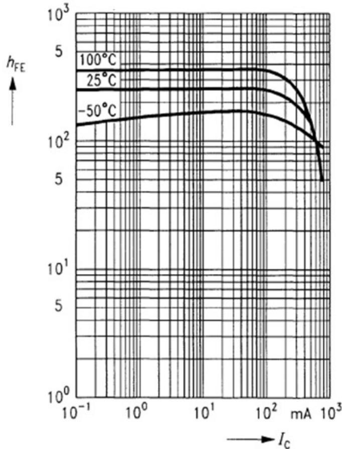
Fig. 4.3.2. Variation of the  $H_{FE}$  amplification factor as a function of the collector current for a DC BC817 transistor [32].
