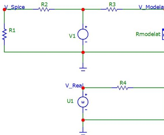
Fig. 3.3.4. Resistive divider made in SPICE.
