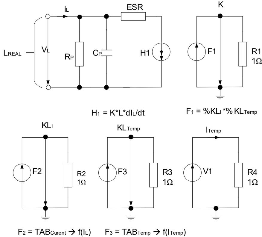
Fig. 3.2.2. SPICE model of a real nonlinear current-controlled coil.
