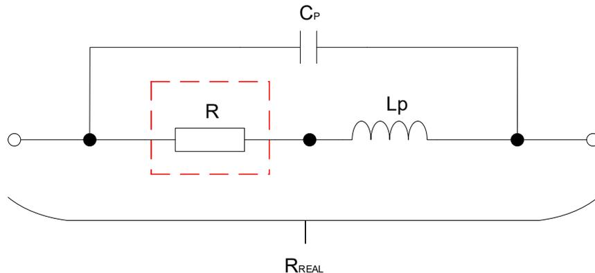
Fig. 3.3.1. The equivalent circuit of a real resistor.
