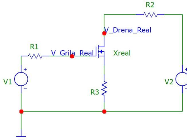
Fig. 4.4.3. Practical circuit for the study of the "n" channel MOS-FET transistor (IRFH3707).
