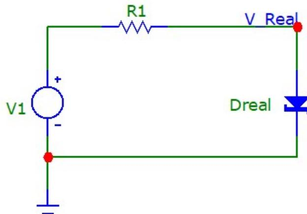
Fig. 4.2.6. Voltage drop across a real Zener diode - practical circuit.
