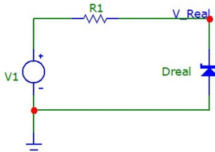
Fig. 4.2.3. Voltage drop across a real stabilizer diode - practical circuit.
