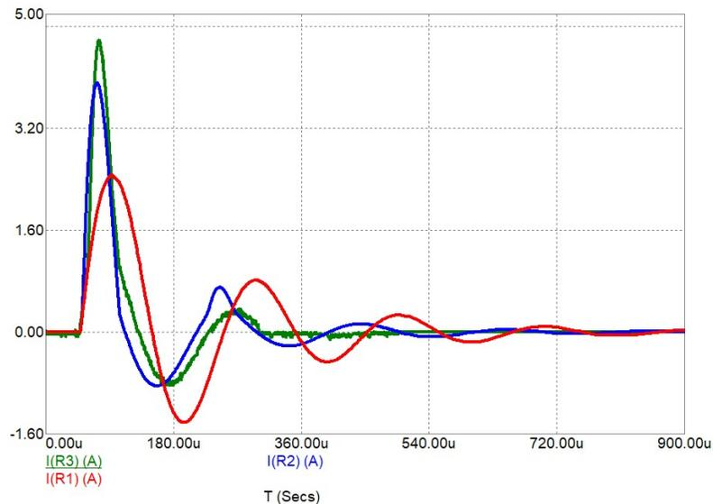
Fig. 3.2.5. Time variation of current through a real coil compared to a nonlinear model modeled in SPICE and a SPICE model in an oscillating circuit.
