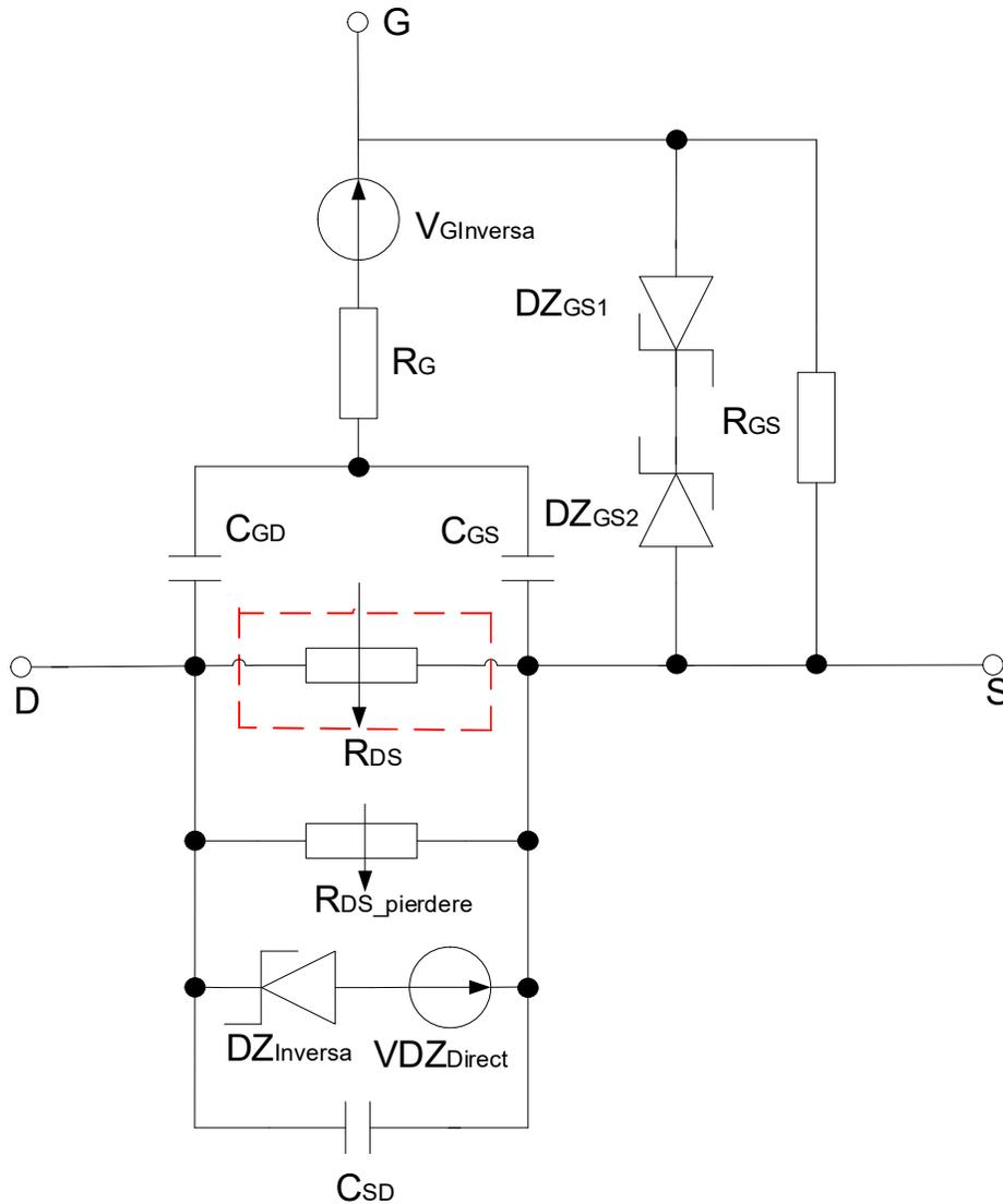
Fig. 4.4.1. The equivalent circuit of a real MOS-FET transistor.
