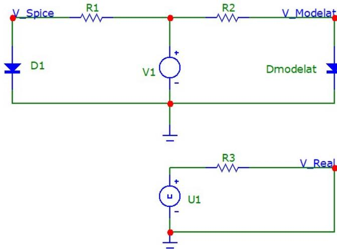
Fig. 4.1.4. Voltage drop across a diode (modeled in SPICE, SPICE, Real) – circuit made in SPICE.
