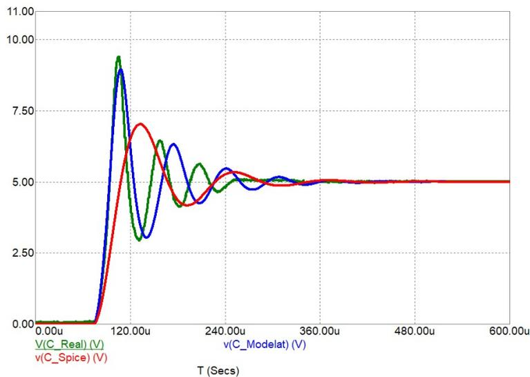
Fig. 3.1.9. Time variation of the voltage of a real capacitor compared to a nonlinear model modeled in SPICE and a SPICE model in an oscillating circuit.
