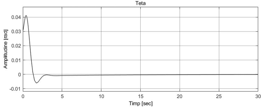
Figure 13: Teta output for  $\theta_{ref} = 0 \text{ rad}$  and  $\theta_0 = 0.03 \text{ rad}$
