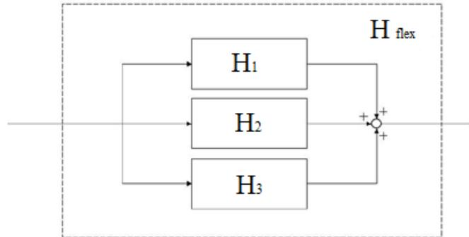
Figure 5: Block diagram of flexible modes
