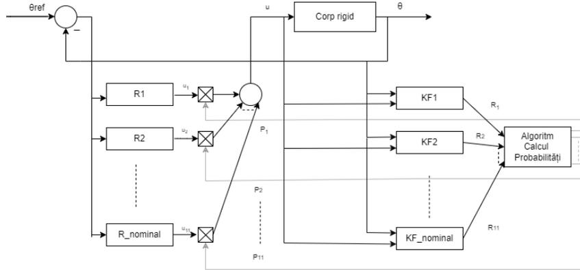
Figure 6: RMMAC control scheme
