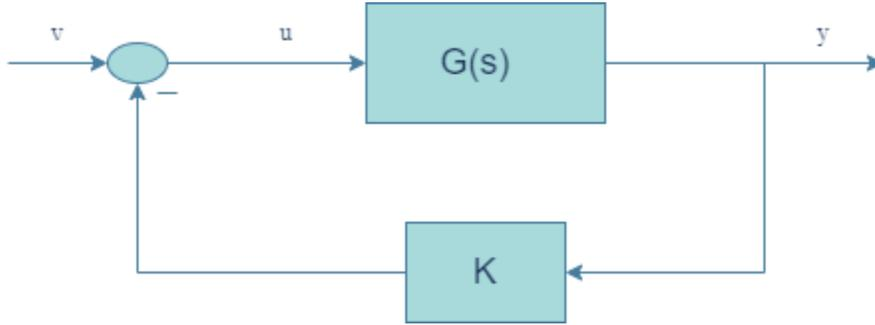
*Figure 10: Closed-loop system*
