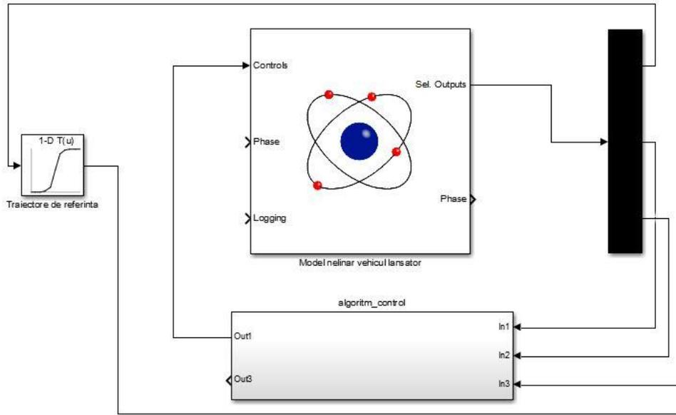
Figure 15: Control algorithm in Simulink using non-linear model
