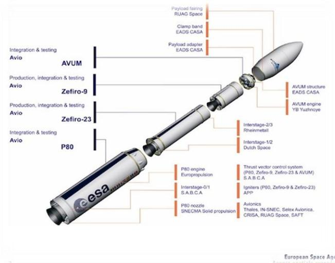
Figure 1: Vega Launcher components [<http://www.esa.int/esapub/br/br257/br257.pdf>]
