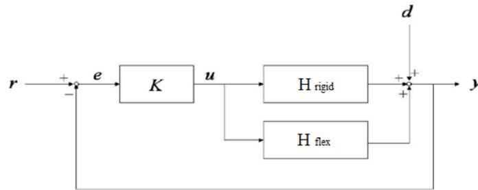
Figure 4: Block diagram of rigid body and flexible modes
