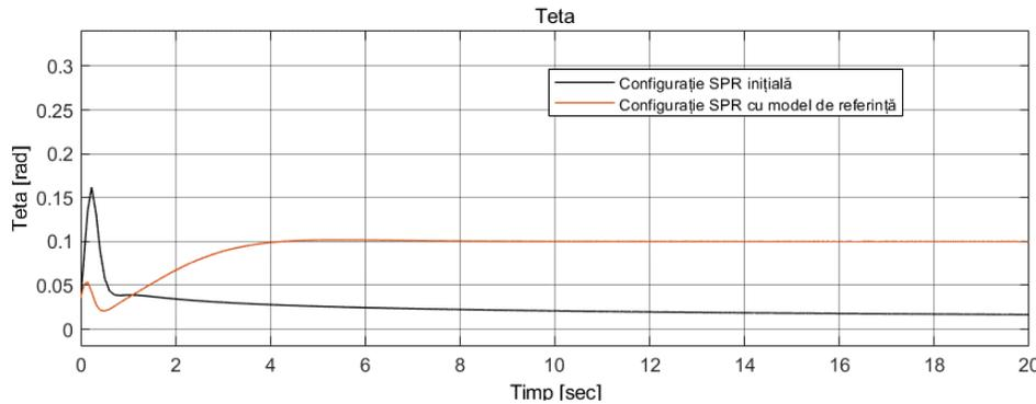
Figure 14: Teta output for  $\theta_{ref} = 0.1 \text{ rad}$  and  $\theta_0 = 0.03 \text{ rad}$
