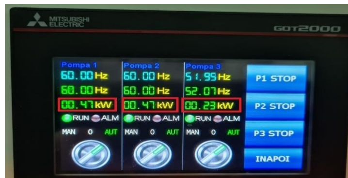
Fig. 4.6. Ecran HMI: puterile electrice absorbite de motoare, P_{elmas1} \div P_{elmas3} [kW]
