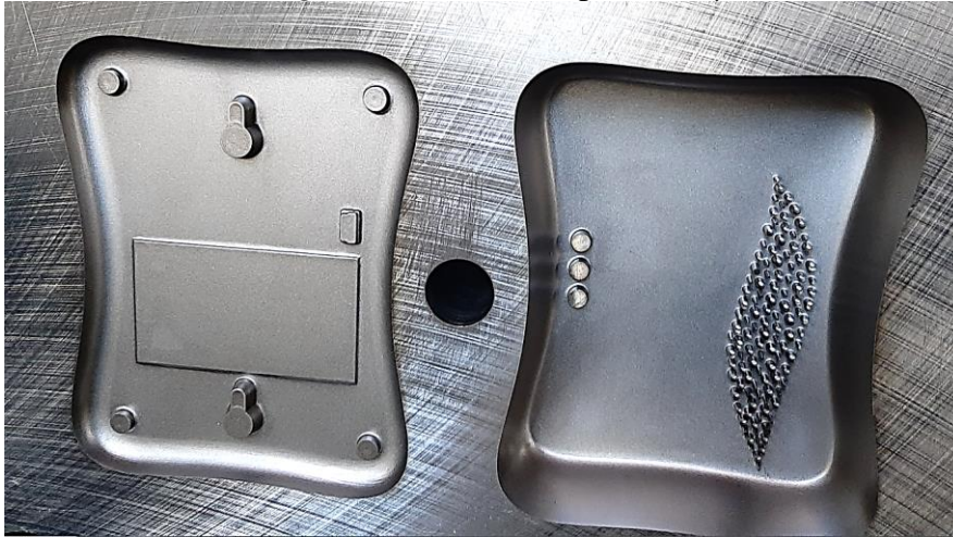
Fig. 5.47 EDM texturing VDI 3400 #22, courtesy LS INTEH srl.
