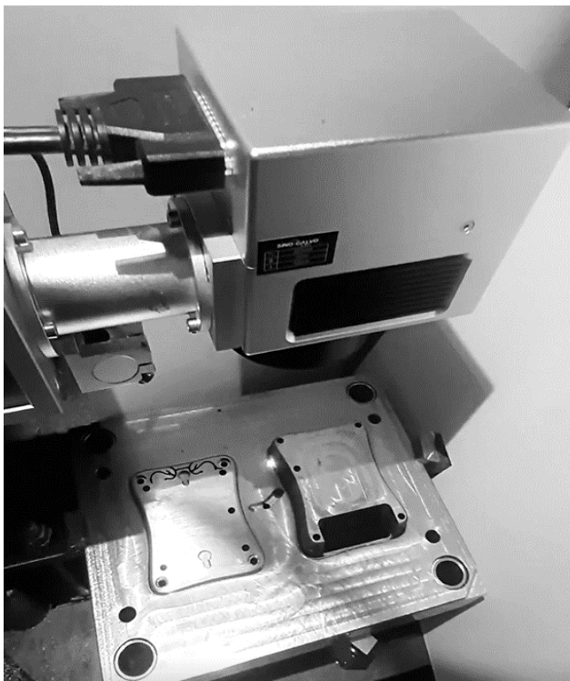
Fig. 6.27 Complex system – laser pocket milling steel DIN 1.2714
