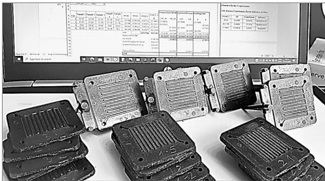
Fig. 7.1 The bipolar plates injection molded in PP87GR (model shown in Fig. 6.9a)
