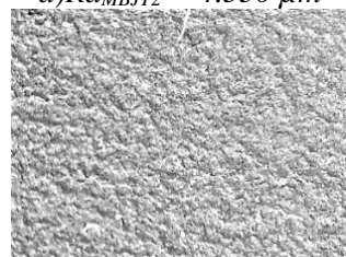
c) Ra_{IM37-MBJT2} = 4.148 \mu\text{m} rRa = 91.5\% \Delta = 0.381 \mu\text{m}
