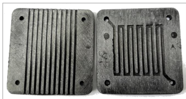
Fig. 8.10 Injection Molded Bipolar Plates, sample nr. 27 cathodes, nr. 26 anodes (C3 recipe)
