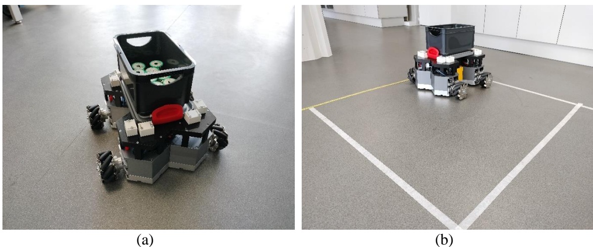
Fig. 0.48 Physical trajectory and real mobile robot with four mecanum wheels: (a) close-up view; (b) mobile robot on trajectory.
