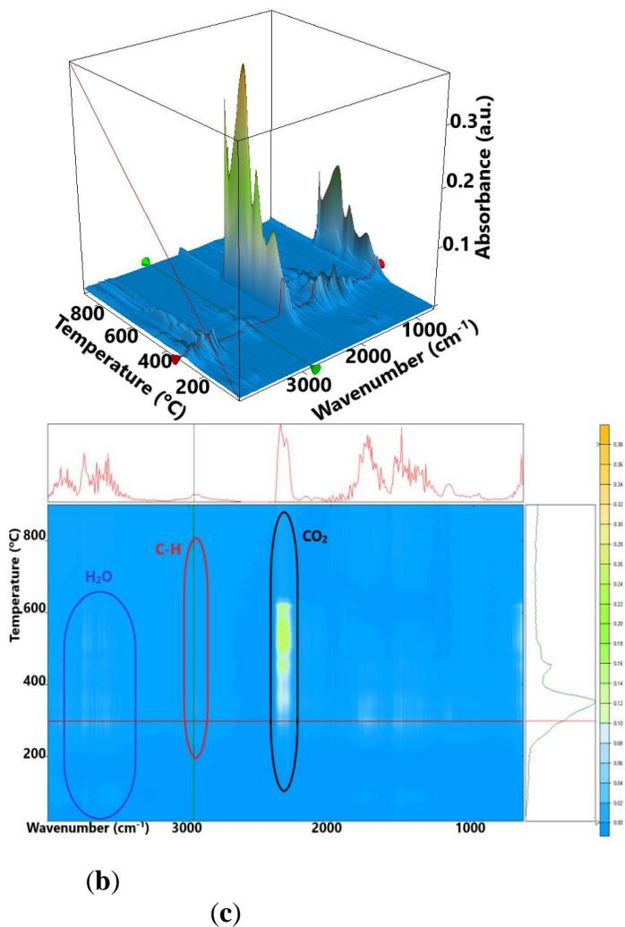
**Figure 11.** Thermal characteristics of the chitosan-sulfonated ethylene-propylene-diene terpolymer membranes (Chi-sEPDM) (M2): (a) thermal diagram, (b) 3D complex analysis; (c) 2D complex analysis.
