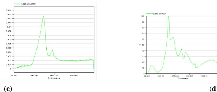
**Figure 12.** Trace for evolving (a)  $\text{SO}_2$  ( $1367 \text{ cm}^{-1}$ ); (b)  $\text{CO}_2$  ( $2355 \text{ cm}^{-1}$ ); (c) hydrocarbons ( $2964 \text{ cm}^{-1}$ ); and (d)  $\text{H}_2\text{O}$  ( $3566 \text{ cm}^{-1}$ ) vs temperature.
