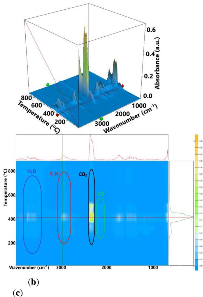
**Figure 9.** Thermal characteristics of the sulfonated ethylene-propylene-diene terpolymer (sEPDM) membrane (M1): (a) thermal diagram; (b) 3D complex analysis; (c) 2D complex analysis.
