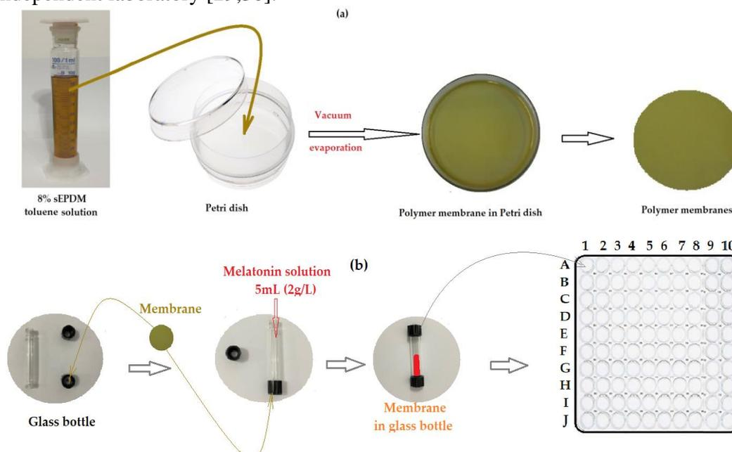
**Figure 3.** Schematic representation of the procedure for obtaining sEPDM based membranes (a); and release schematic procedure (b).
