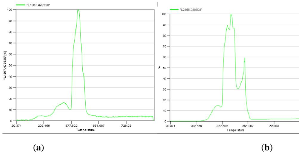
**Figure 10.** Trace for evolving  $\text{SO}_2$  ( $1367\text{ cm}^{-1}$ ) vs temperature (a); and trace for evolving  $\text{CO}_2$  ( $2355\text{ cm}^{-1}$ ) vs temperature (b).
