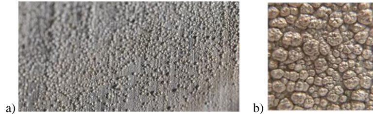
Figure 8.48. Technical details (reverse) in which the pure silver layer is electrolytically deposited (colloidal silver) is observed on the copper matrix.
