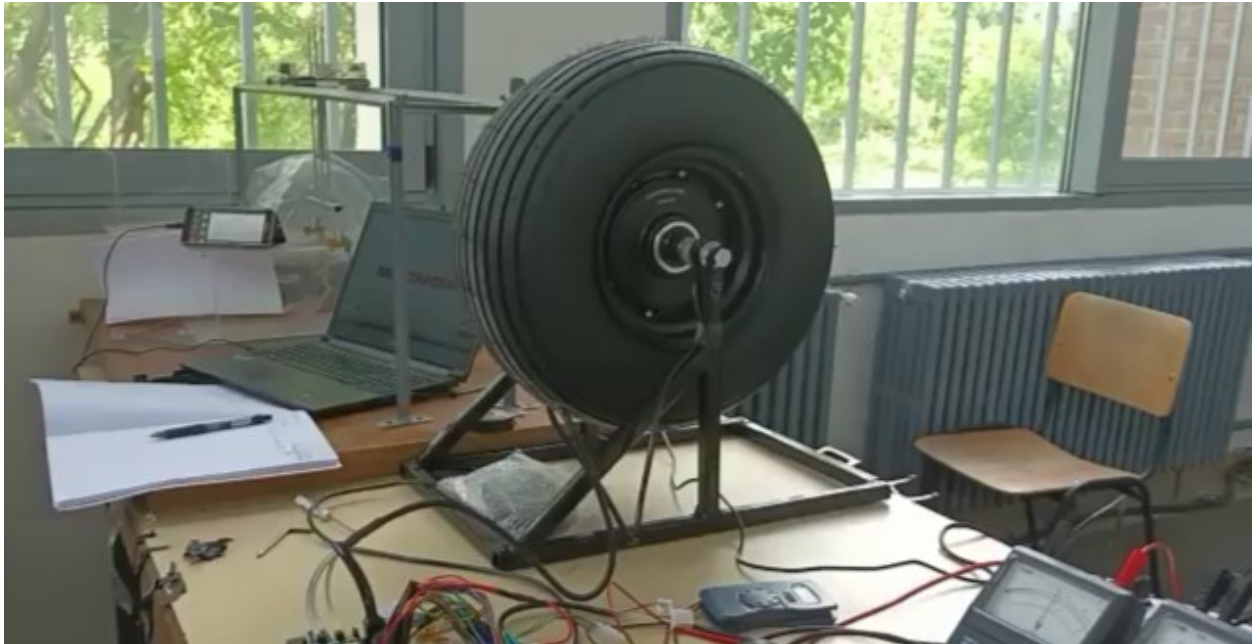
Fig. VIII-1. Physical platform integrating one single motor
