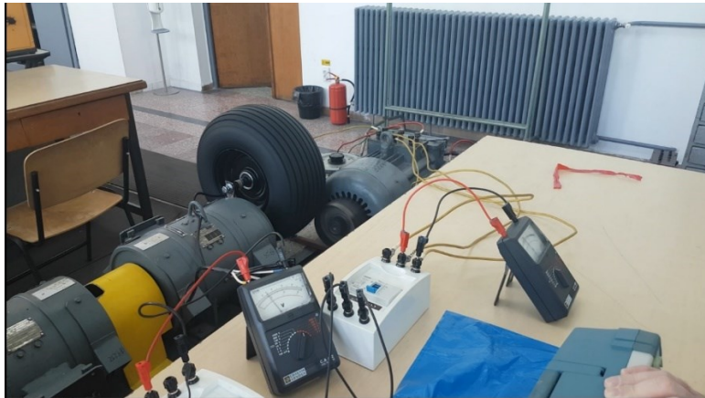
Fig. VIII-9. Running the PM motor as a generator for firsts determinations
