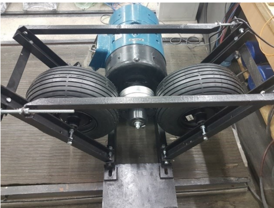
Fig. VIII-2. Platform with two in-wheel motors – image on coupling between wheels
