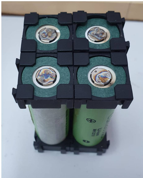
Figure 13.2. Battery consisting of 4 lithium-ion batteries mounted in parallel
