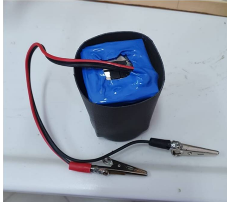
Figure 13.3. Lithium-ion battery pack with attached connectors
