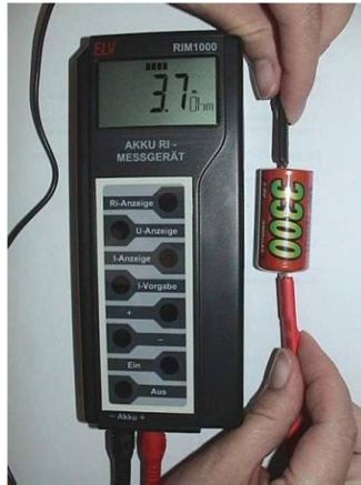
Figure 5.1. Ohmmeter for measuring the internal resistance of batteries
