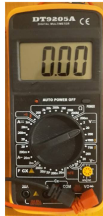
Figure 5.2. DT9205A digital multimeter
