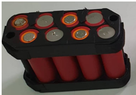
Figure 13.4. Group of eight revitalized batteries
