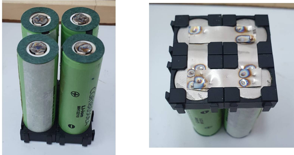
Figure 13.1. MH12210 lithium-ion batteries equipped with modular coupling systems and insulating rings to prevent accidental short circuits
