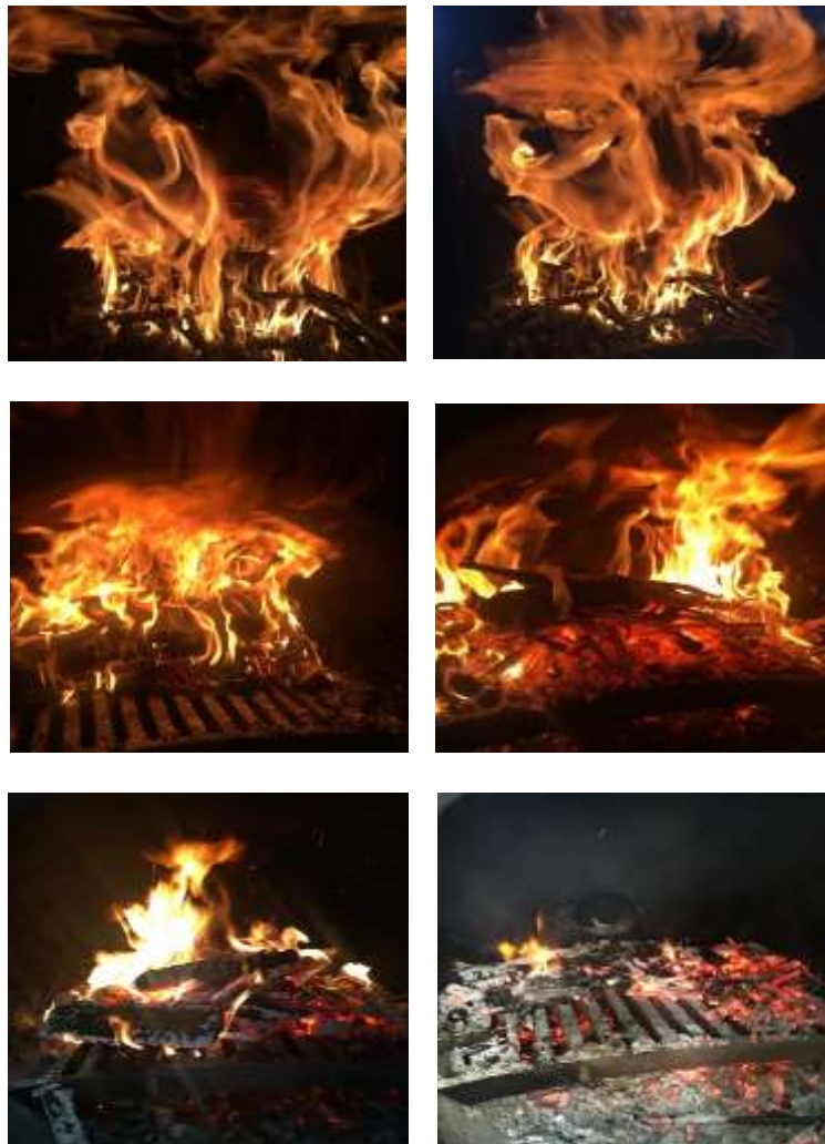
Fig. 9. Images of the combustion process inside the hearth of the 55 kW pilot boiler at different times of experiment 1
