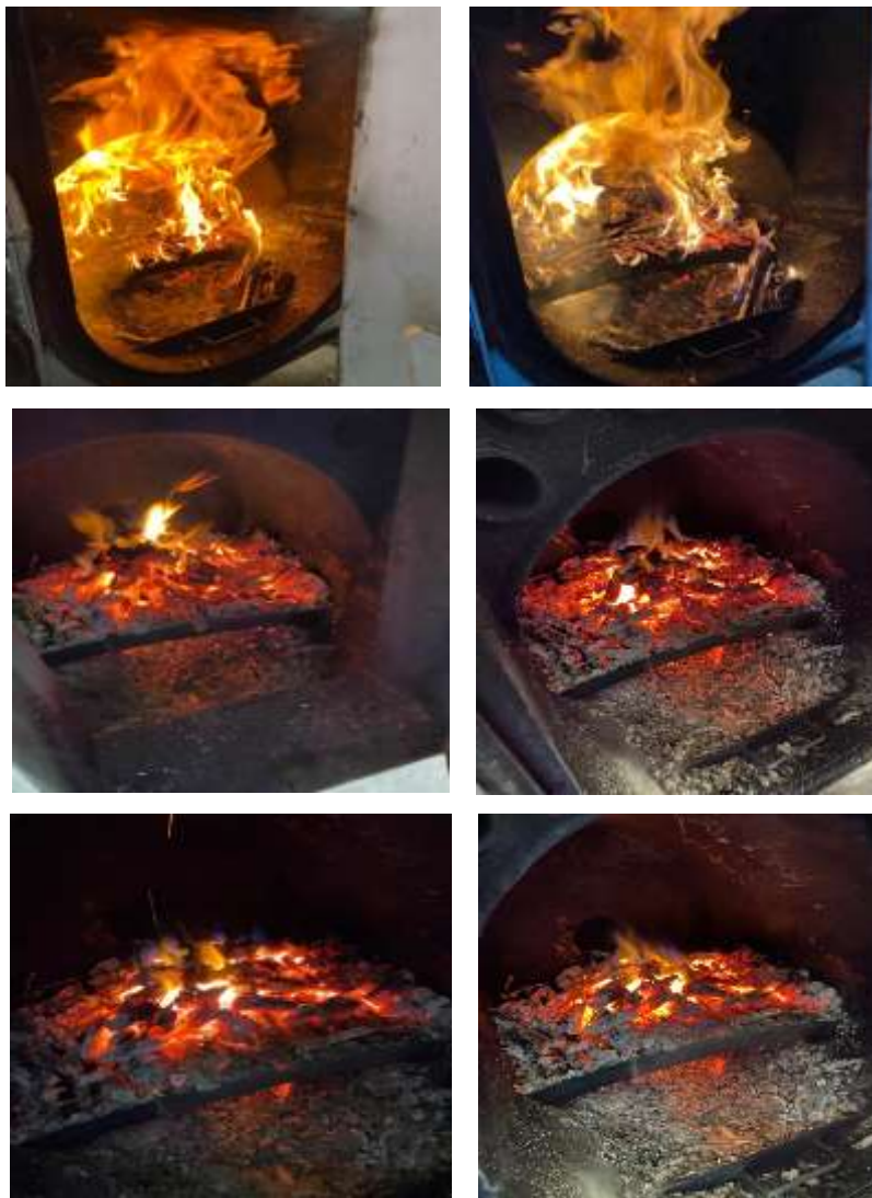
Fig. 11. Images of the combustion process inside the hearth of the 55 kW pilot boiler at different times of experiment 2
